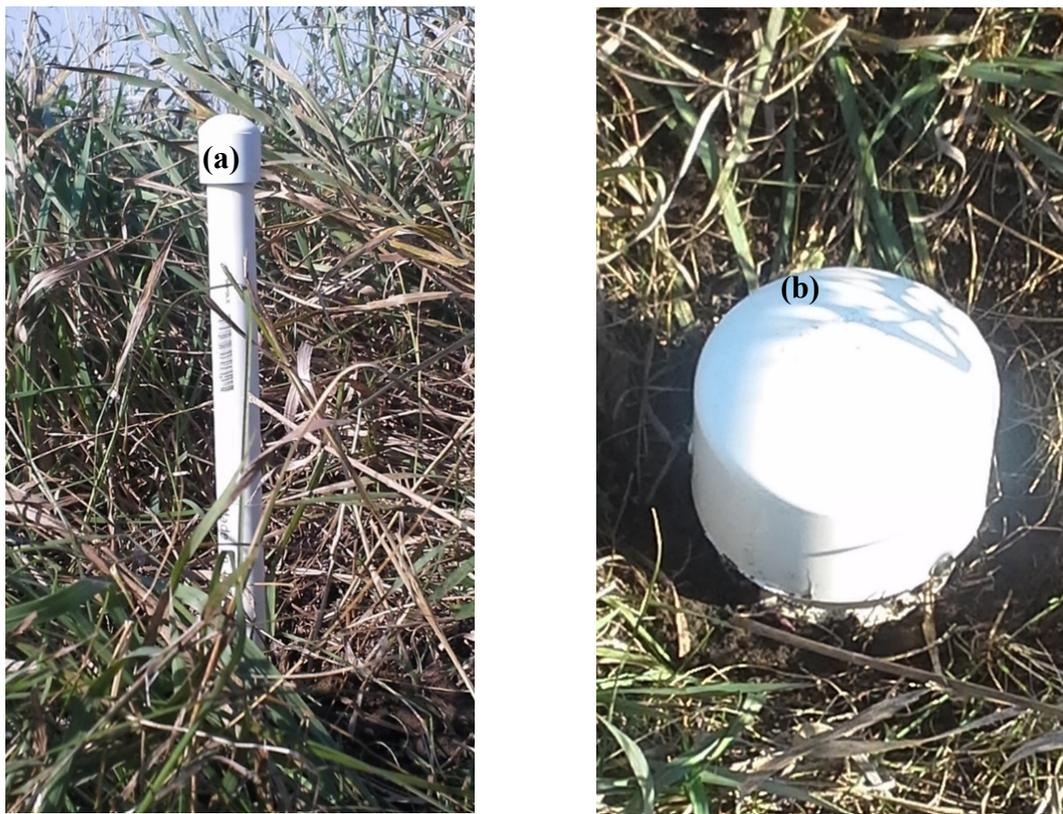
**Figure 2.** Leachate sampling well in roadside ditches (a) during installation and (b) after installation.
