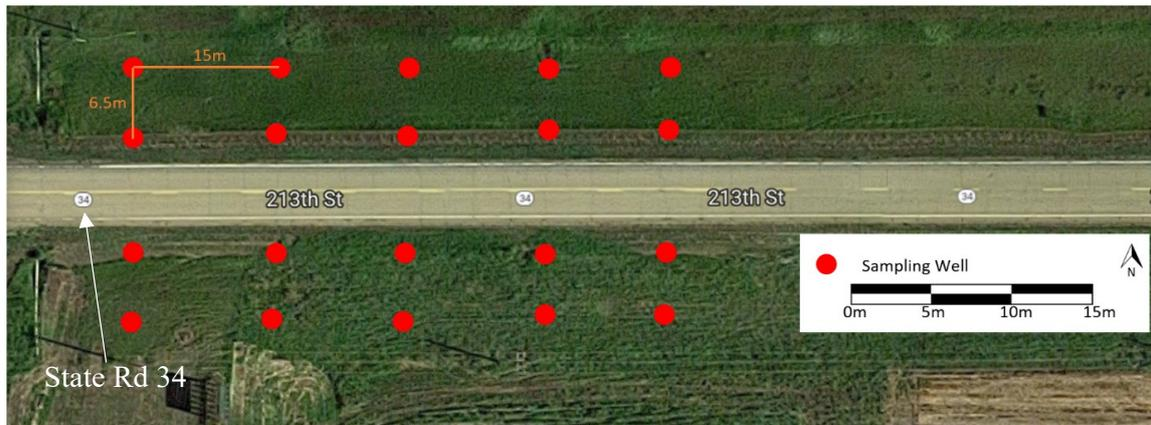
**Figure 3.** Schematic diagram of leachate sampling locations in roadside ditches during this study in South Dakota.
