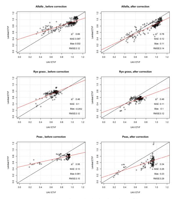
**Figure 10.** Change of ETrF with and without the application of the time series integration factor on alfalfa, rye grass, and peas. Each subplot represents the scatterplot with the corresponding coefficient of determination, mean absolute error, bias, and root mean square values. Black line is the line with slope of 1 and red line is the line of regression.
