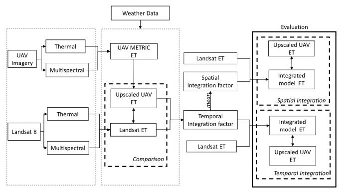
**Figure 3.** Flowchart for the comparison and integration of ET. Integrated model ET is the combination of the Landsat and UAV ET.
