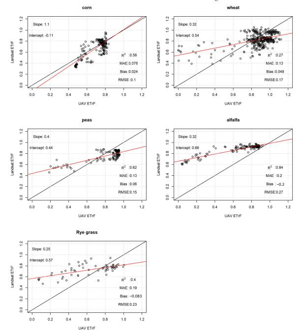
**Figure 6.** Scatterplot of Landsat ETrF vs. UAV EtrF on five sample crops used for this study. Each subplots represent the scatterplot with the corresponding slope, intercept, coefficient of determination, mean absolute error, bias, and root mean square error values. Black line is the line with slope of 1 and red line is the line of regression.
