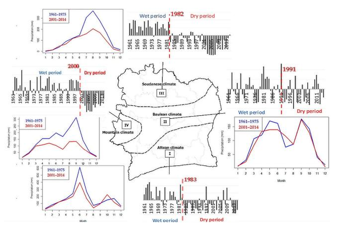
**Figure 5.** Break detection and reduced centered index in annual precipitation (PRCPTOT) from 1961 to 2015 in each climate area. The annual cycles in the subperiods before (1961–1975) and after (2001–2014) the break are plotted in blue and red, respectively.
