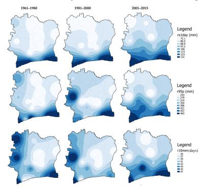
**Figure 3.** Spatial variability of 1-day maximum annual precipitation (RX1 DAY on the **top row**), intense rainfall (R95 P on the **middle row**), and rainy days with a 10 mm threshold (R10 mm on the **bottom row**) for the periods of 1961–1980 (**bottom column**) for the periods of 1961–1980 (**left column**), 1981–2000 (**middle column**), and 2001–2015 (**right column**).
