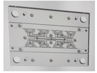
Figure 1. Cold runner injection mold type.
