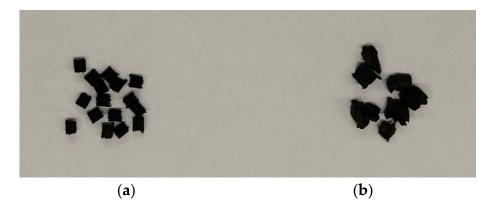
Figure 3. Virgin polyamide granules (a) regrind from runner systems waste (b).
