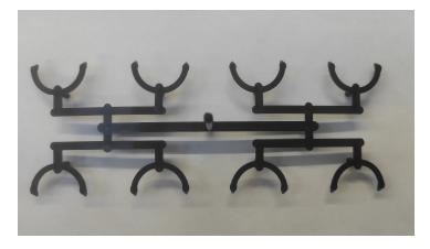
Figure 2. The characteristic waste of a runner in a cold runner system.
