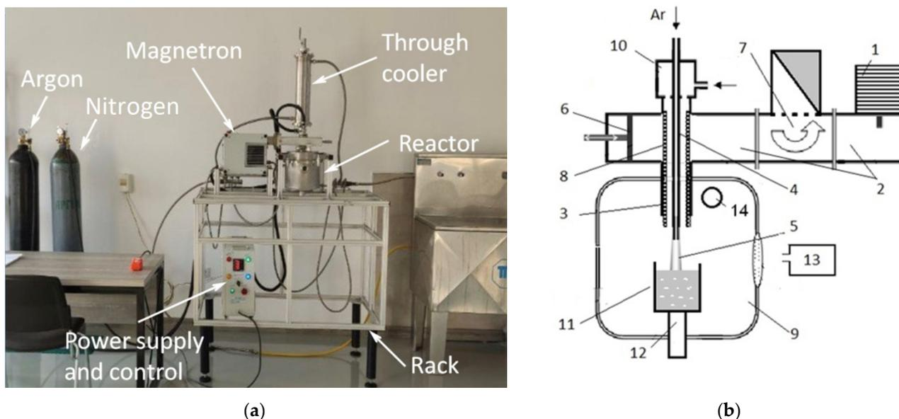
**Figure 1.** (a) Photography of the installation during operation; (b) the installation diagram; 1 magnetron, 2 rectangular waveguides, 3 coaxial waveguides, 4 copper tubes, 5 plasma torches, 6 pistons for adjusting the microwave path, 7 circulators, 8 quartz tubes, 9 reactor chambers, 10 mixers, 11 containers with water, 12 movable rods, 13 spectrometers, 14 outlet pipes.
