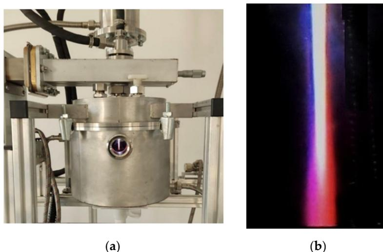
**Figure 2.** Argon microwave discharge torch, which leads to the activation of aqueous solutions placed in the reactor chamber: (a) In general view, the torch is visible in the viewing window of the reactor; (b) magnified photography of the torch (real scale).
