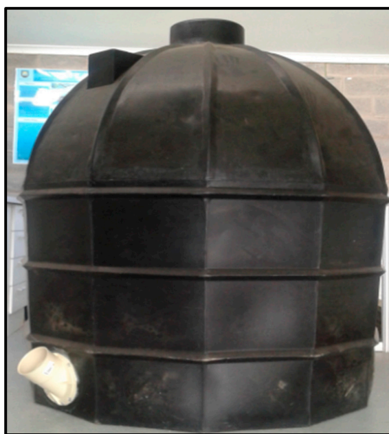
Figure 1. Fabricated high-density polyethylene biogas digester.
