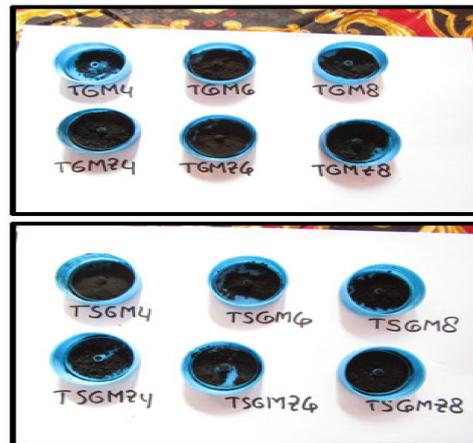
**Figure 8.** Products of CNS (code without Z) and ZnO/CNS nanocomposites (code with Z) which were resulted from evaporation of the colloids of the carbon prepared from sawdust (SG) and rice husk (G).
