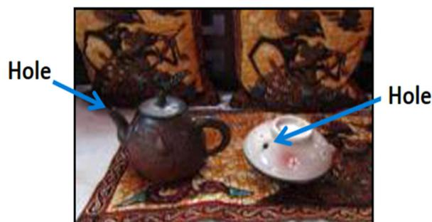
**Figure 2.** Earthenware for pyrolysis and ceramics ware for calcination by microwave.
