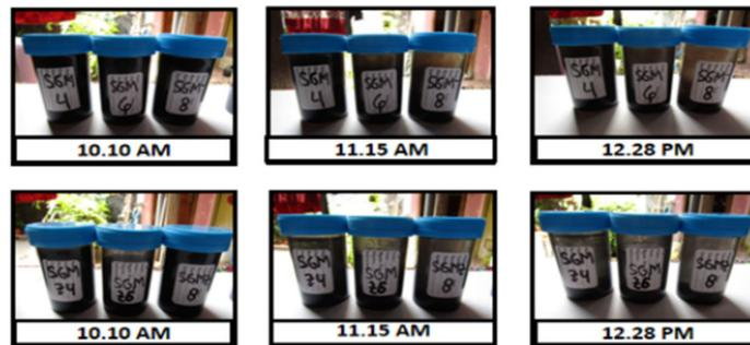
**Figure 16.** Colloid stability of CNS from pyrolysis of sawdust (SG) without  $ZnCl_2$  (SMG) and  $ZnO/CNS$  from pyrolysis of sawdust (SG) with  $ZnCl_2$  (SGMZ).
