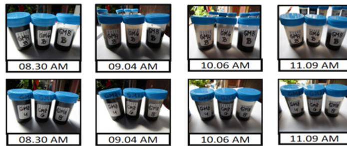
**Figure 15.** Colloid stability of CNS from pyrolysis of the rice husk (G) without  $ZnCl_2$  (without Z) and  $ZnO/CNS$  from pyrolysis of rice husk (G) with  $ZnCl_2$  (with Z).
