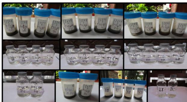
**Figure 21.** Residues and filtrates after test of pesticide degradation.
