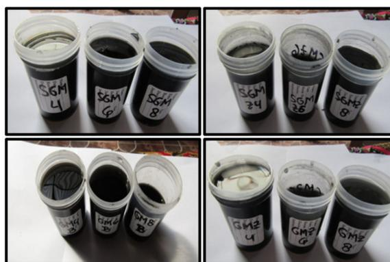
**Figure 7.** Concentrated colloid of CNS (code without Z) and ZnS/CNS (code with Z) which were prepared from pyrolysis of sawdust (SG) and rice husk (G).
