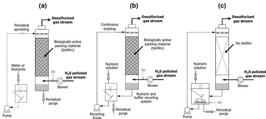
**Figure 3.** Biofiltration unit configurations: (a) Biofilter; (b) biotricking filter (BTF); (c) Bioscrubber.
