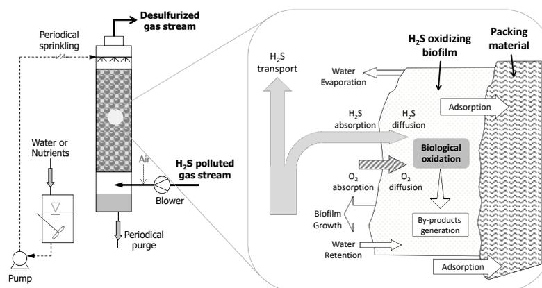
**Figure 4.** Schematic representation of the complex interactions that take place in biofilters.
