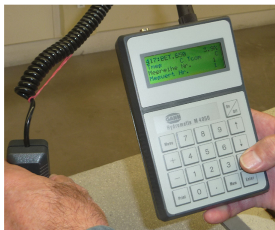
Figure 1. Measurement of the surface humidity in a nondestructive way via the Gann-device.
