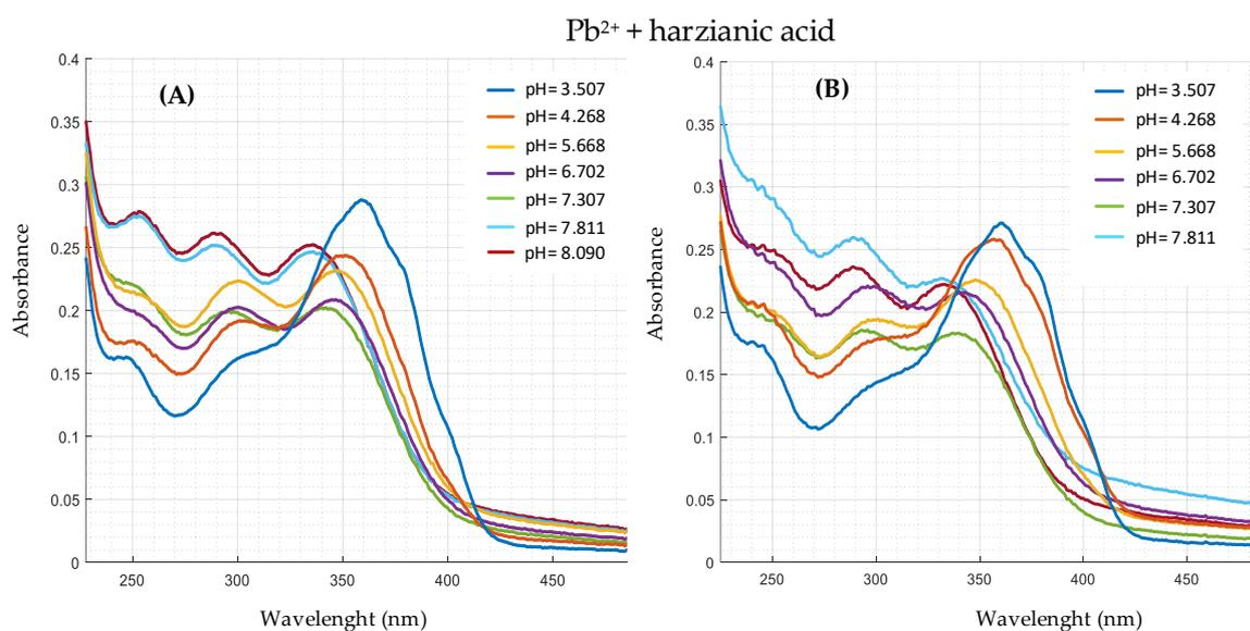
**Figure 6.** UV-VIS spectra in CH<sub>3</sub>OH/0.1 M NaClO<sub>4</sub> (50:50 *w/w*) at different pH of: (A) C<sub>H<sub>2</sub>L</sub><sup>0</sup> = 2.0 × 10<sup>−4</sup> M and C<sub>Pb</sub><sup>0</sup> = 2.0 × 10<sup>−4</sup> Pb(ClO<sub>4</sub>)<sub>2</sub> (ligand to metal ratio 1:1); (B) C<sub>H<sub>2</sub>L</sub><sup>0</sup> = 2.0 × 10<sup>−4</sup> M and C<sub>Pb</sub><sup>0</sup> = 4.0 × 10<sup>−4</sup> Pb(ClO<sub>4</sub>)<sub>2</sub> (ligand to metal ratio 1:2).
