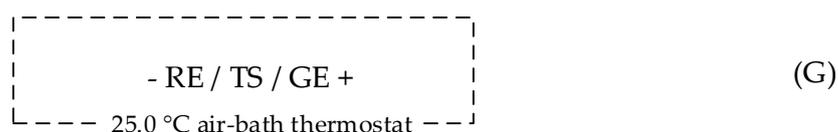
**Scheme 1.** Sketch of the potentiometric apparatus employed to prepare test solutions, TS, of accurately known pH and analytical composition. RE represents the double junction  $Ag/AgCl(s)/0.1\text{ M NaCl}/(0.1\text{ M NaClO}_4\text{-}CH_3OH, 50/50\text{ }w/w)$  reference electrode and GE a pH indicator glass electrode.
