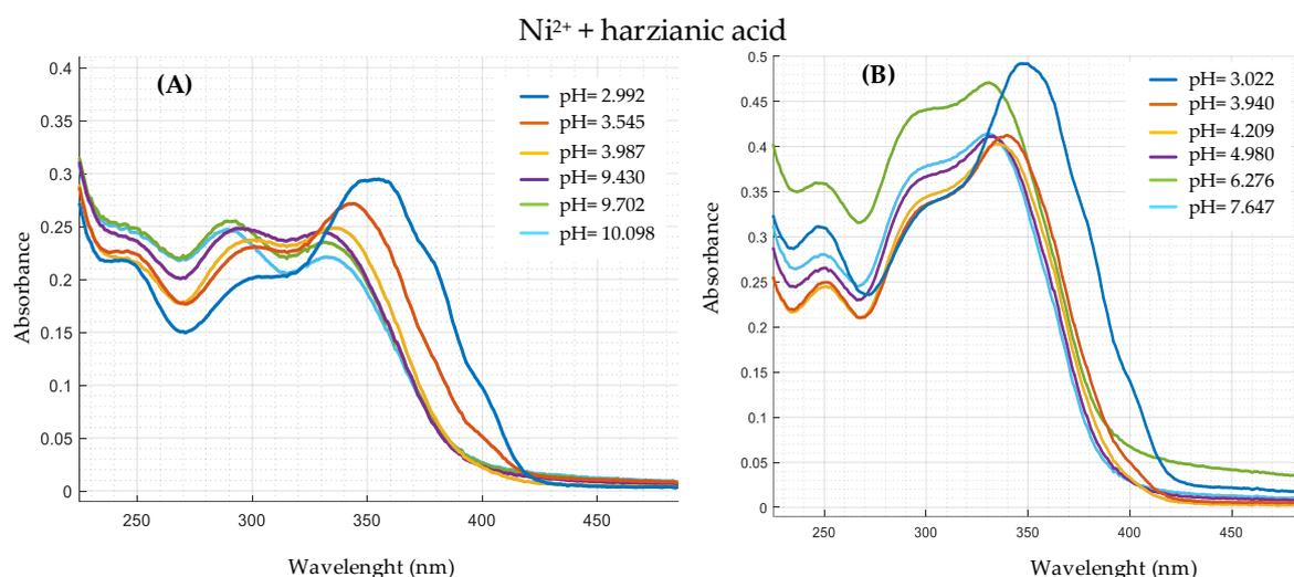
**Figure 5.** UV-VIS spectra in CH<sub>3</sub>OH/0.1 M NaClO<sub>4</sub> (50:50 *w/w*) at different pH of: (A) C<sub>H<sub>2</sub>L</sub><sup>0</sup> = 2.0 × 10<sup>−4</sup> M and C<sub>Ni</sub><sup>0</sup> = 2.0 × 10<sup>−4</sup> NiCl<sub>2</sub> (ligand to metal ratio 1:1); (B) C<sub>H<sub>2</sub>L</sub><sup>0</sup> = 2.0 × 10<sup>−4</sup> M and C<sub>Ni</sub><sup>0</sup> = 4.0 × 10<sup>−4</sup> NiCl<sub>2</sub> (ligand to metal ratio 1:2).
