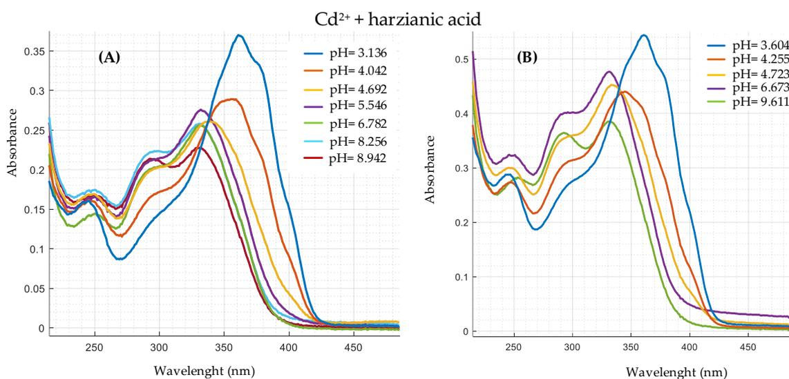
**Figure 3.** UV-VIS spectra in  $\text{CH}_3\text{OH}/0.1$  M  $\text{NaClO}_4$  (50:50  $w/w$ ) at different pH of: (A)  $C_{\text{H}_2\text{L}}^0 = 2.0 \times 10^{-4}$  M and  $C_{\text{Cd}}^0 = 2.0 \times 10^{-4}$   $\text{Cd}(\text{ClO}_4)_2$  (ligand to metal ratio 1:1); (B)  $C_{\text{H}_2\text{L}}^0 = 2.0 \times 10^{-4}$  M and  $C_{\text{Cd}}^0 = 4.0 \times 10^{-4}$   $\text{Cd}(\text{ClO}_4)_2$  (ligand to metal ratio 1:2).
