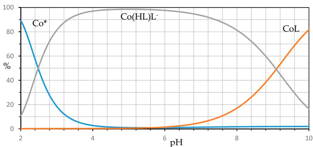
**Figure 10.** Distribution diagram of species in  $Co^{2+}$ -harzianic acid system in  $CH_3OH/0.1\text{ M NaClO}_4$  (50:50 *w/w*) calculated from formation constants in Table 2 assuming  $C_{Co} = 1.0 \times 10^{-3}\text{ M}$  and  $C_{H_2L} = 2.0 \times 10^{-3}\text{ M}$  ( $H_2L$  = harzianic acid). The symbol  $Co^*$  is used to represent all species in the solution that contain the metal cation, but do not contain harzianic acid.
