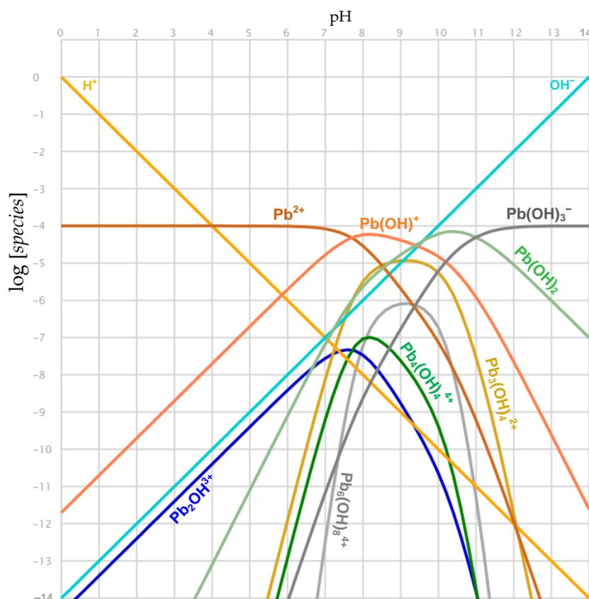
**Figure 7.** pH scan of a  $10^{-4}$  M aqueous solution of  $Pb^{2+}$  based on stoichiometry and formation constants of  $Pb_m(OH)_n^{2m-n}$  hydroxo complexes gathered from literature [45,46].
