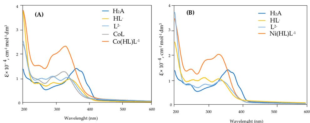
**Figure 8.** Molar extinction coefficients,  $\epsilon_\lambda (\text{M}^{-1}\text{cm}^{-1})$ , of the absorbing species calculated by Hyperquad for the systems: (A)  $\text{Co}^{2+}$ -harzianic acid; (B)  $\text{Ni}^{2+}$ -harzianic acid.
