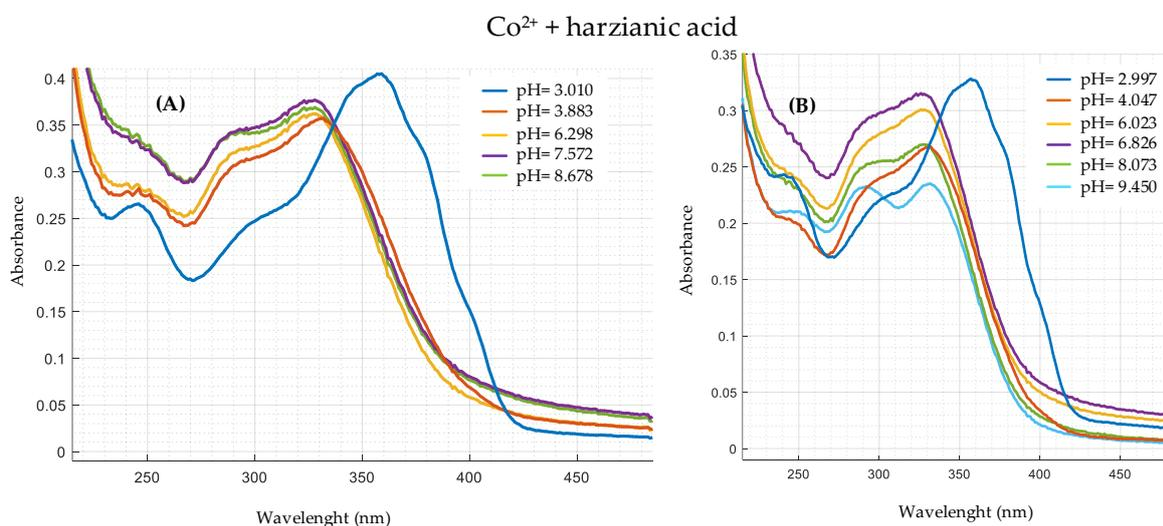
**Figure 4.** UV-VIS spectra in  $\text{CH}_3\text{OH}/0.1$  M  $\text{NaClO}_4$  (50:50  $w/w$ ) at different pH of: (A)  $C_{\text{H}_2\text{L}}^0 = 2.0 \times 10^{-4}$  M and  $C_{\text{Co}}^0 = 2.0 \times 10^{-4}$   $\text{CoCl}_2$  (ligand to metal ratio 1:1); (B)  $C_{\text{H}_2\text{L}}^0 = 2.0 \times 10^{-4}$  M and  $C_{\text{Co}}^0 = 4.0 \times 10^{-4}$   $\text{CoCl}_2$  (ligand to metal ratio 1:2).
