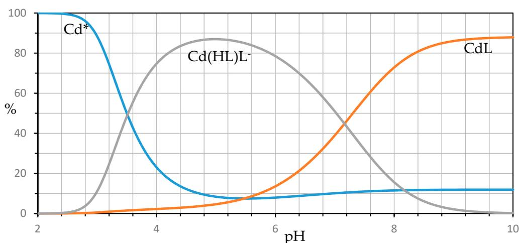
**Figure 9.** Distribution diagram of species in  $Cd^{2+}$ -harzianic acid system in  $CH_3OH/0.1\text{ M NaClO}_4$  (50:50 *w/w*) calculated from formation constants in Table 2 assuming a  $C_{Cd} = 1.0 \times 10^{-3}\text{ M}$  and  $C_{H_2L} = 2.0 \times 10^{-3}\text{ M}$  ( $H_2L$  = harzianic acid). The symbol  $Cd^*$  is used to represent all species in the solution that contain the metal cation, but do not contain harzianic acid.
