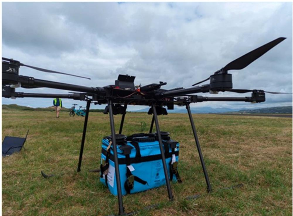
**Figure 8.** Hexacopter drone with bag to be mounted via attached harness.
