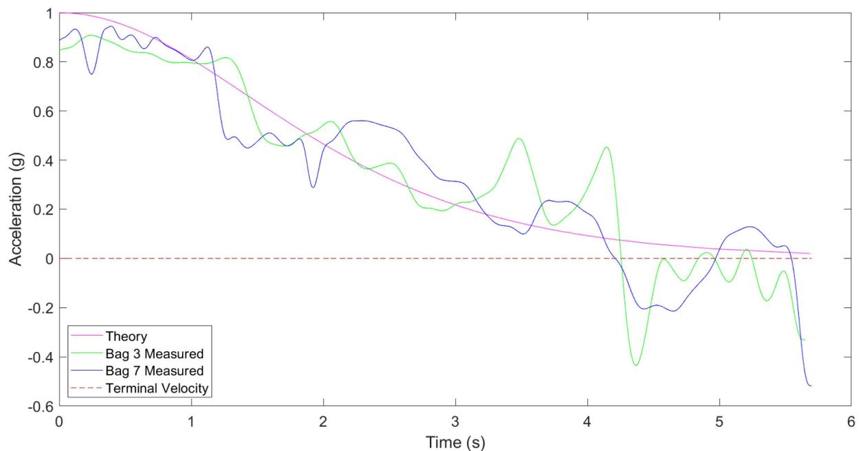
**Figure 11.** Measured and theoretical accelerations during drops.
