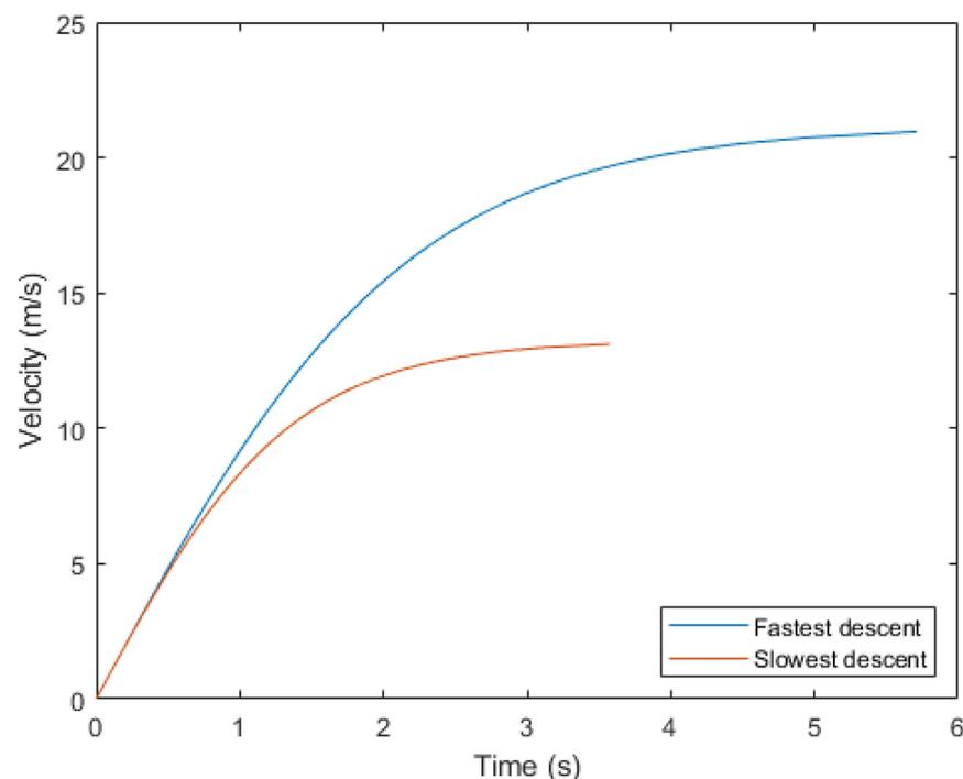
**Figure A1.** Velocity/time curves, with end point representing 99% of terminal velocity.
