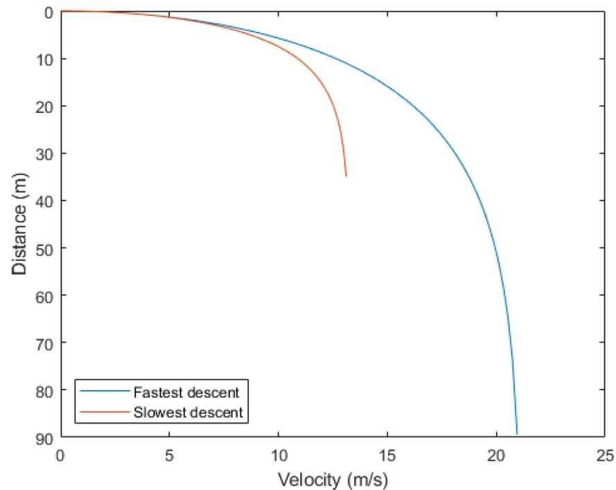
**Figure A2.** Distance (height)/velocity curves, with end point representing 99% of terminal velocity.
