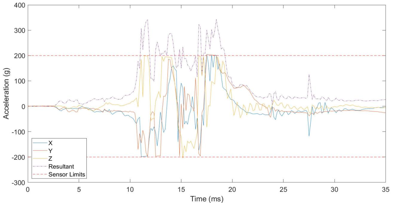
**Figure 10.** Acceleration levels during impact for drop test 4.
