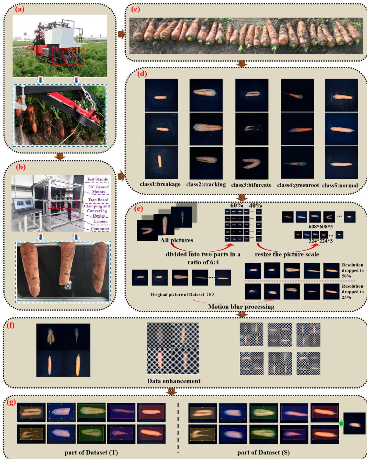
**Figure 3.** Acquisition of a carrot dataset. (a) Operation of the carrot combine harvester conveying system; (b) combine harvesting and collecting simulation system; (c) material acquisition for field tests; (d) classification of carrot defect types; (e) image preprocessing and dataset partitioning; (f) data enhancement; (g) partial dataset demonstration.
