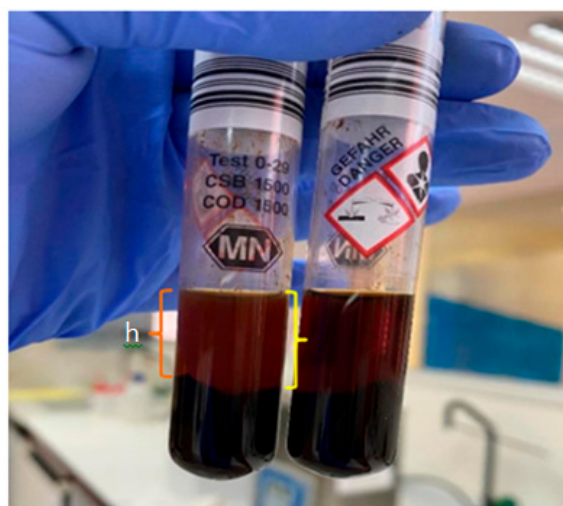
Figure 1. Extraction with acetone at 20% ( m/m ) (right) and 40% ( m/m ) (left): extract (upper phase) and SCG (lower phase).
