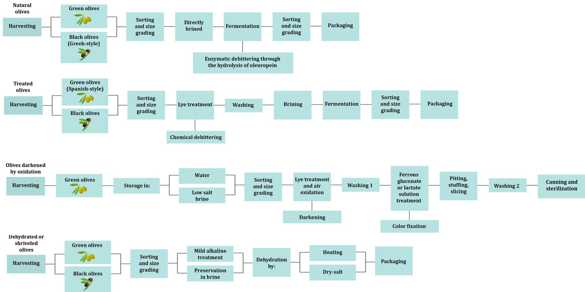
Figure 1. Table olive processing methods.
