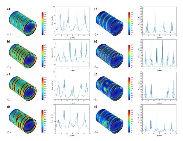
**Figure 3.** Shear rate contour map of fluid in the barrel under different screw elements ((**a1**,**a2**) C-A, (**b1**,**b2**) C-B, (**c1**,**c2**) C-C and (**d1**,**d2**) C-D).
