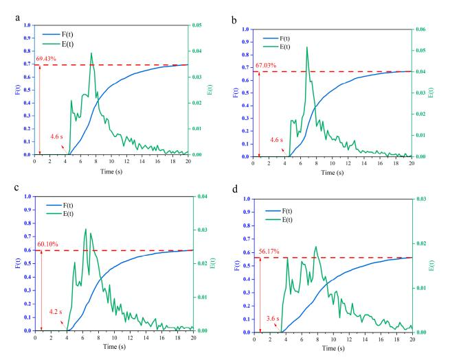
**Figure 7.** Particle residence time distribution inside the barrel for different screw configurations ((a) C-A, (b) C-B, (c) C-C and (d) C-D).
