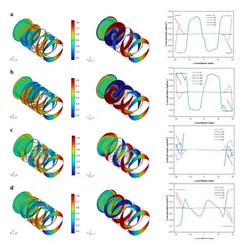
**Figure 8.** Particle residence time distribution in the barrel for different screw configurations ((**a**) C-A, (**b**) C-B, (**c**) C-C and (**d**) C-D).
