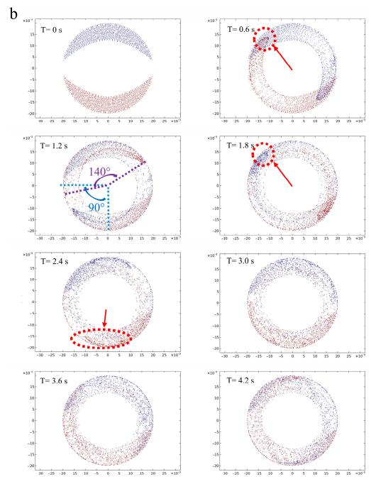
**Figure 5.** Phase diagram of the screw with the kneading block ((**a**) C-C) and reversing elements ((**b**) C-D) with different times.
