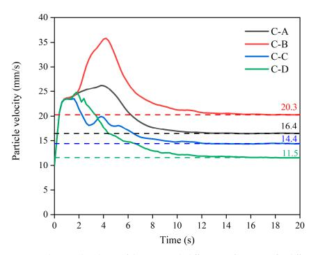
Figure 6. The particle velocity of the screw with different configurations for different times.
