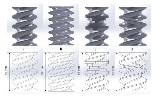
**Figure 1.** The screw model of different screw combinations: conveying (**a**,**b**), kneading block (**c**), and reversing elements (**d**).
