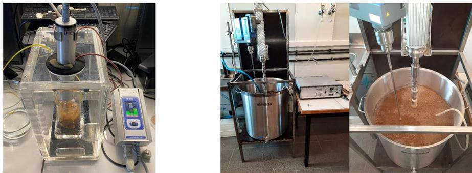
**Figure 1.** Ultrasound setup at lab scale (left) and at pilot scale (right).
