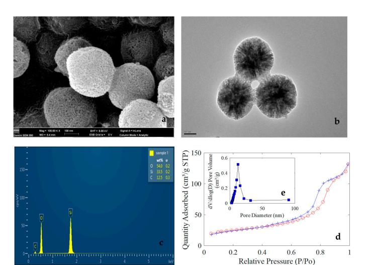
**Figure 3.** The SEM image of MSNs (**a**), TEM image of MSNs (**b**), EDS image of MSNs (**c**), adsorption-desorption hysteresis lines of MSNs (**d**), and the pore size distribution of MSNs (**e**).
