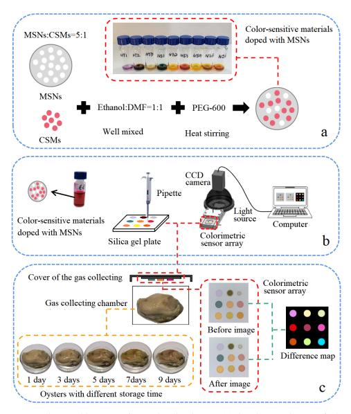
**Figure 1.** The assembly process of CSMs doped with MSNs (**a**), the schematic diagram of colorimetric sensor array system (**b**) and the difference map acquisition of oysters (**c**).
