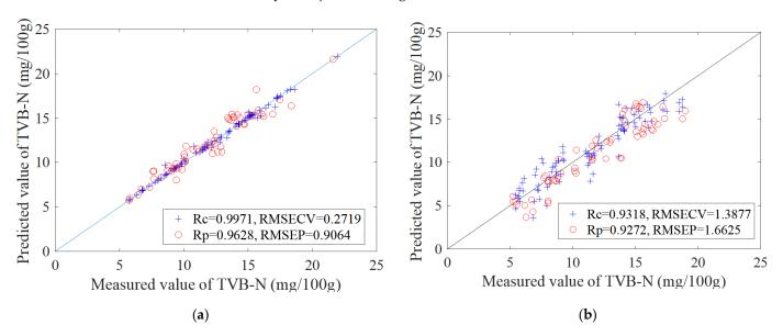
**Figure 6.** TVB-N correlation between Kjeldahl nitrogen-measured values and the prediction value by color-sensitive materials doped with MSNs (**a**); and color-sensitive materials without MSN doping (**b**).
