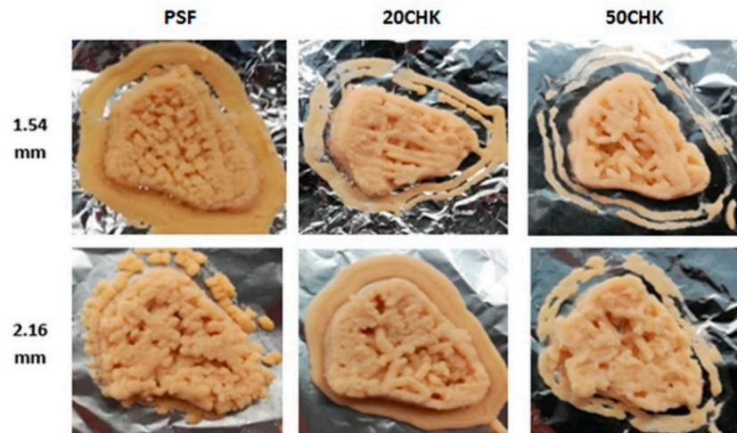
**Figure 6.** Printed meat analogues using 1.54 and 2.16 mm nozzles (15 mm/s, 100% infill). PSF represents PPI paste containing both starch and fat; 20CHK represents 20% chicken added into PSF paste; 50CHK represents 50% chicken added into PSF paste.
