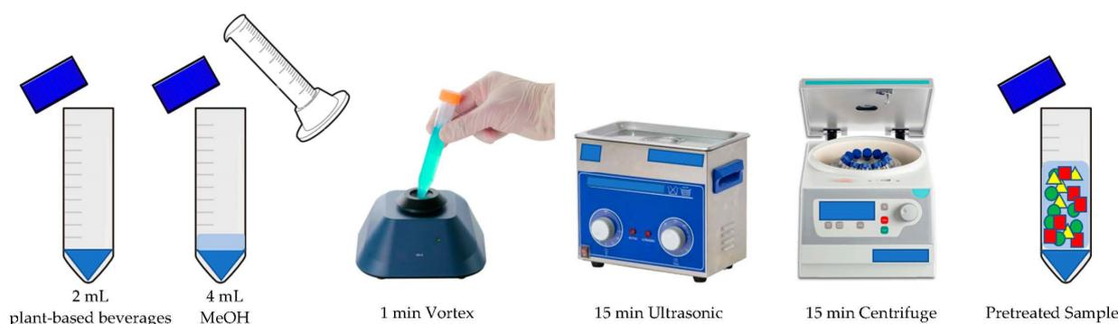
**Figure 1.** Drawing of sample pretreatment process.
