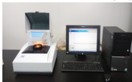
B: SupNIR-2700 grating NIR spectrometer
