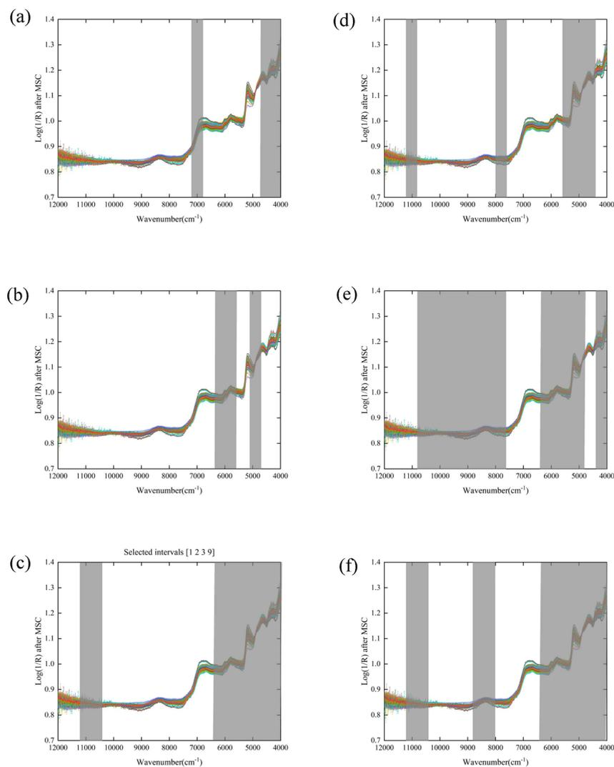
**Figure 3.** The optimization of spectral intervals, developed by siPLS and biPLS algorithm for quality compounds: (a) siPLS for TP; (b) siPLS for FAA; (c) siPLS for TP/FAA; (d) biPLS for TP; (e) biPLS for FAA; (f) biPLS for TP/FAA.
