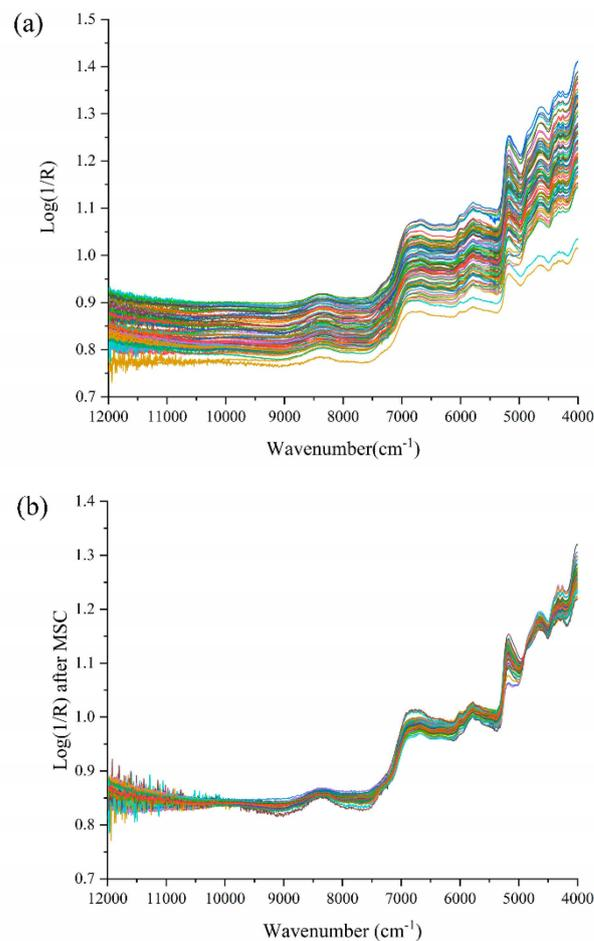
**Figure 1.** The spectra of all tea samples in the wavenumber range of 12,000–4000  $\text{cm}^{-1}$ . (a) original spectra ( $\log 1/R$ ); (b) spectra after pretreatment by multiplicative signal correction (MSC).
