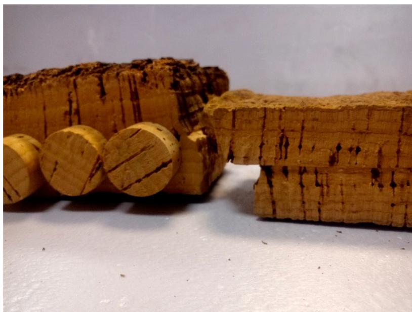
**Figure 1.** Perforated cork sheet to obtain one-piece stoppers on the left and 2 thin cork sheets glued together to achieve the same useful thickness and manufacture two-piece stoppers on the right.
