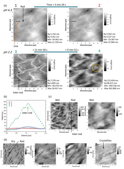
**Figure 1.** In situ AFM analysis of human enamel. (a) Time-lapse of AFM images showing the AFM height profiles of enamel during exposure to different pH 4.3 and 2.2, and the measurement of Rq, Ra and the minimum and maximum of the height reported. (b) Height line profile analysis from the locations in (a) highlighted with orange arrow on the first image, and (c) AFM analysis at a lower and higher magnification in a wet condition, and (d) in a dry condition.
