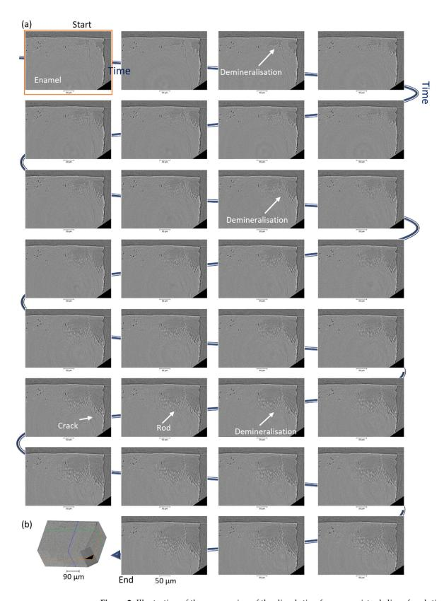
**Figure 2.** Illustration of the progression of the dissolution from one virtual slice of each time point tomogram. (a) Virtual slices in xy axis, from the first time point  $t_0$  to the last time point  $t_{end}$  (scale bar 50  $\mu$ m), and (b) 3D view with the highlight of the plane displayed, data non-filtered, additional slices from the other axis in Supplementary Materials Figures S7 and S8. The varnish was also visualised on the virtual slices.
