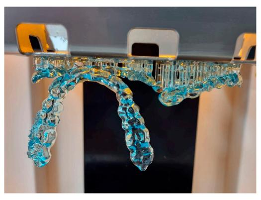
**Figure 5.** Printed splints in  $0^{\circ}$ ,  $30^{\circ}$  and  $90^{\circ}$  orientations (Nextdent 5100).
