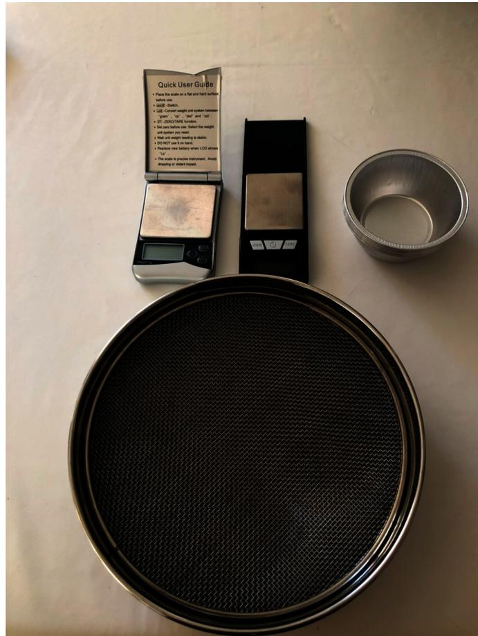
**Figure 1.** Precision scale and sieve used to collect and weight the specimens.
