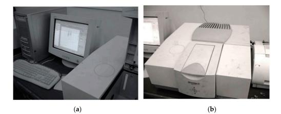
Figure 1. IRPrestige-21, infrared spectrophotometer: (a) desktop computer; (b) interferometer.
