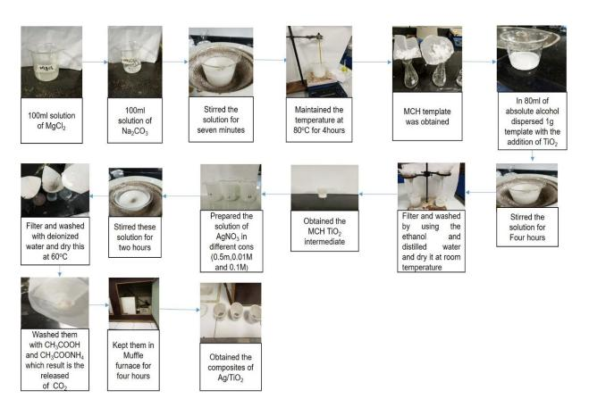
Figure 1. Schematic diagram of the synthesis of Ag/TiO<sub>2</sub> composites by template induced route.
