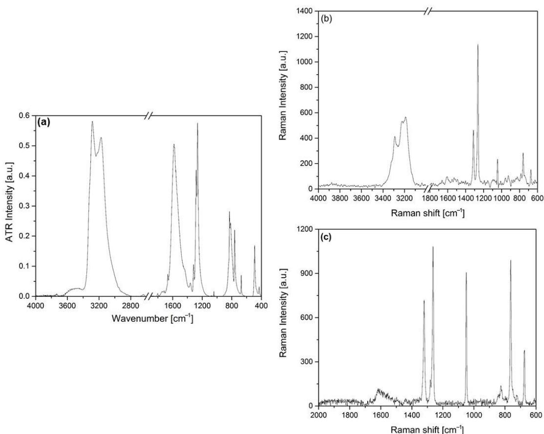
**Figure 5.** The (a) IR (25 °C) and low-temperature Raman spectra ( $-150\text{ }^\circ\text{C}$ ) in the region of (b) the ammonia (532 nm excitation); and (c) carbonate (785 nm excitation) vibrational modes.
