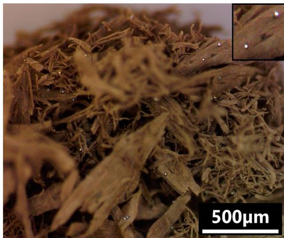
**Figure 7.** Stereomicroscopic image of the small metallic cobalt particles on the surface of CoO particles (magnification 55×).
