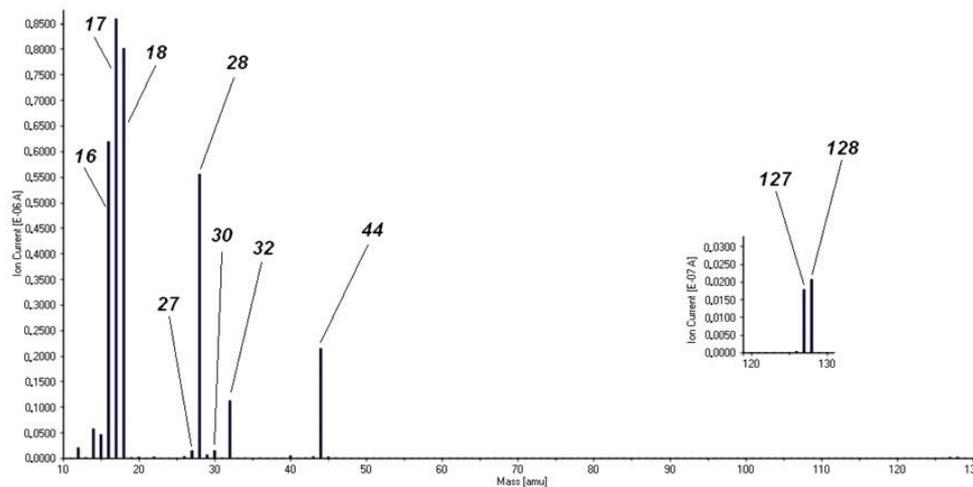
**Figure 10.** Analogous TG-MS spectra of the main gaseous decomposition products of compound 1 (please note that the numbers are representing  $m/z$  data).
