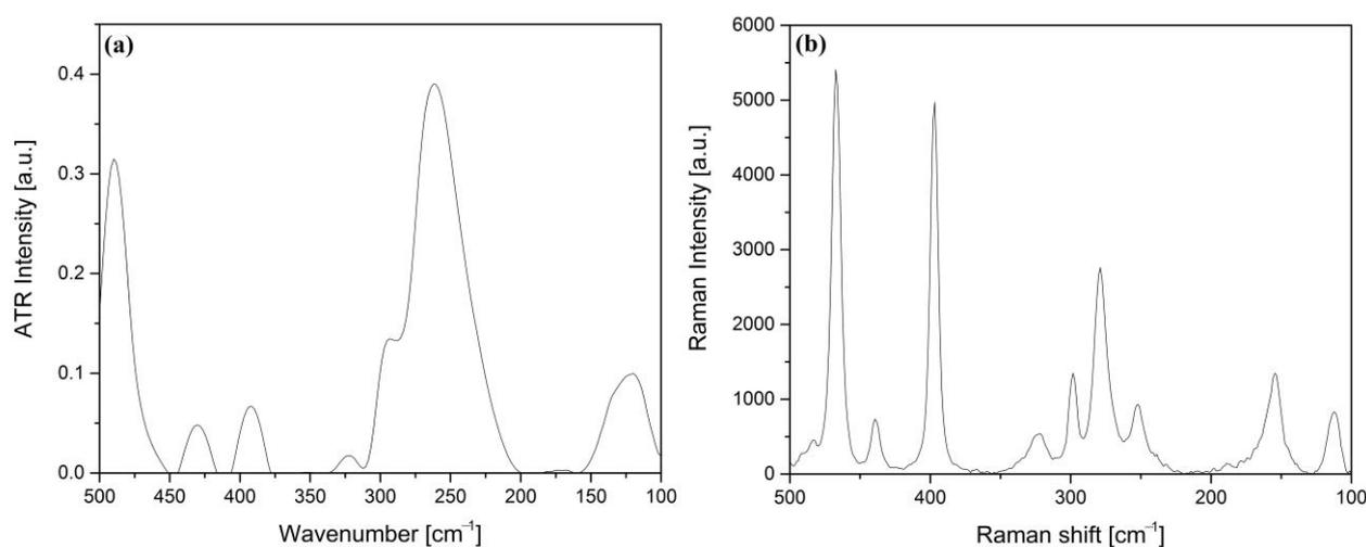
**Figure 4.** (a) The far-IR (25 °C) and (b) low-temperature Raman (785 nm excit., –150 °C) spectra between 500 and 100  $cm^{-1}$ .
