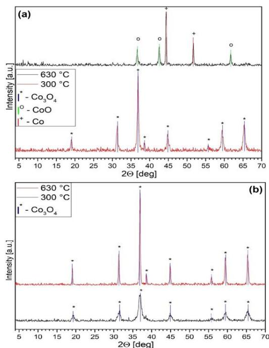
**Figure 8.** XRD of the decomposition products of compound 1 at 300 °C and 630 °C in (a) helium atmosphere and in (b) air.
