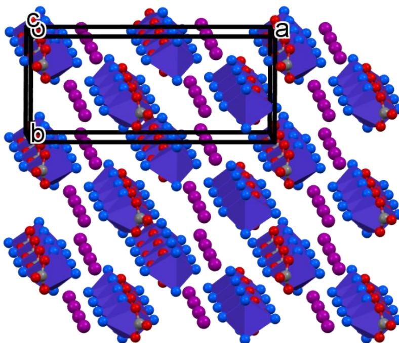
**Figure 2.** Packing arrangement in the crystal lattice of  $[\text{Co}(\text{NH}_3)_4\text{CO}_3]\text{I}$  (a, b, c are axes marks and o is the origin).
