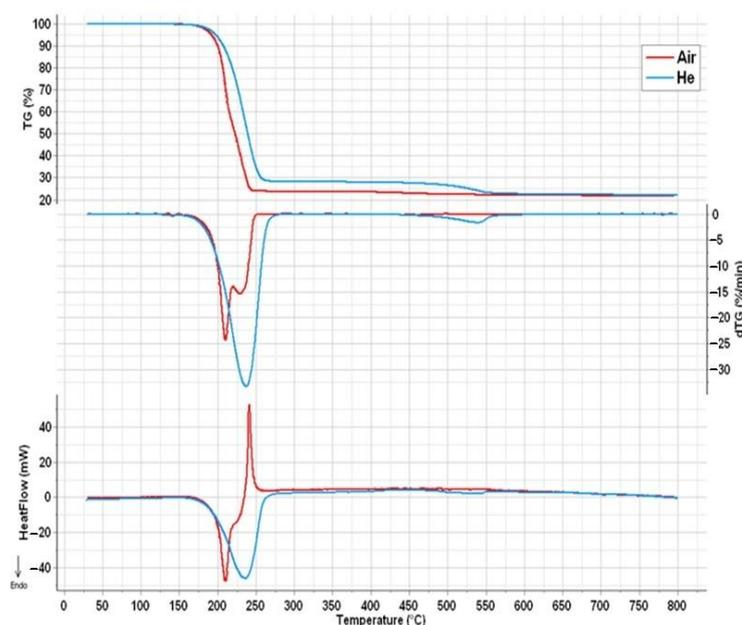
**Figure 6.** The thermal decomposition characteristics of compound **1** in helium atmosphere and in air.
