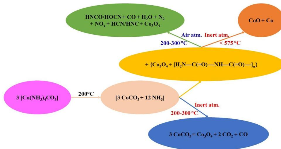
**Scheme 1.** Reaction routes during the thermal decomposition of  $[\text{Co}(\text{NH}_3)_4\text{CO}_3]$ .
