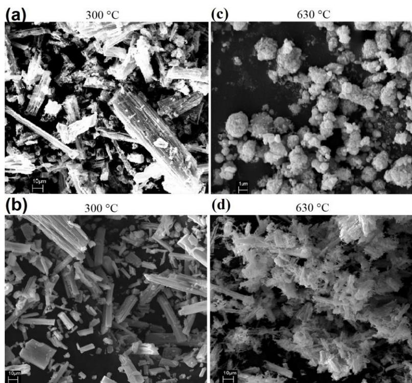
**Figure 9.** The SEM pictures of the decomposition products formed from compound **1** at 300 and  $630\text{ }^\circ\text{C}$ : (a,c) in air, and (b,d) in He atmosphere).
