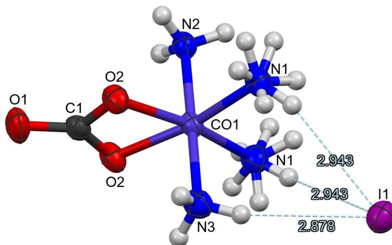
**Figure 1.** Structure of compound 1 at 100 K (thermal ellipsoids are drawn at the 50% probability level, hydrogen bonds between the ammonia ligands and the iodide anion are drawn by blue dashed lines).
