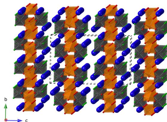
**Figure 3.** Representation of the single crystal structure of  $\text{Rb}_4\text{Ge}_5\text{O}_9\text{F}_6$ . Rubidium atoms are shown in blue,  $\text{GeO}_3\text{F}_3$  octahedra in grey,  $\text{GeO}_4$  tetrahedra in orange, oxygen atoms in red, and fluorine atoms in green.
