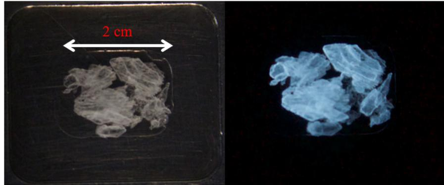
**Figure 5.** Optical images of  $Rb_4Ge_5O_9F_6:Nb$  crystals in the absence of X-rays (left) and of the same crystals scintillating under X-ray excitation (right).
