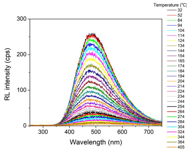
**Figure 6.** Selected RL spectra for  $Rb_4Ge_5O_9F_6:Nb$  up to 405 °C.
