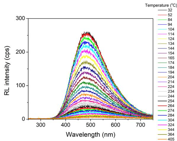
**Figure 6.** Selected RL spectra for  $\text{Rb}_4\text{Ge}_5\text{O}_9\text{F}_6:\text{Nb}$  up to 405 °C.
