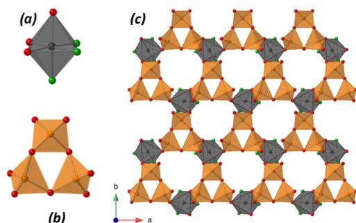
**Figure 2.** Illustration of (a)  $\text{GeO}_3\text{F}_3$  octahedra, (b)  $\text{Ge}_3\text{O}_9$  unit, and (c) their connectivity to form the germanium oxyfluoride layer. Germanium octahedra are shown in grey, germanium tetrahedra in orange, oxygen in red, and fluorine in green.
