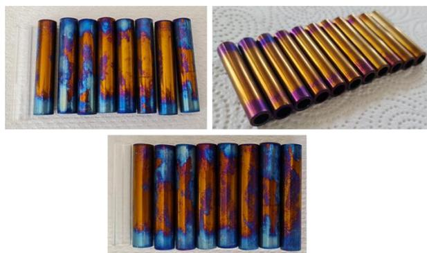
**Figure 14.** Raschig rings after heat treatment.
