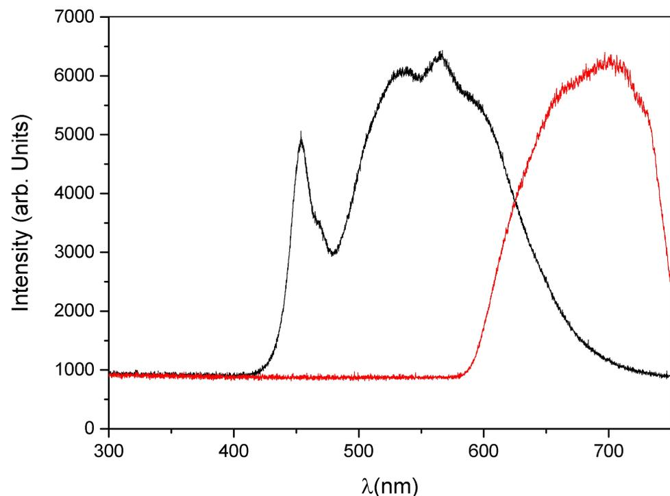
**Figure 1.** Absorption spectra of the incoherent lamps used in our experiments (black line = white LED lamp; red line = NIR lamp). The intensity impinging on the sample is  $\approx 50 \text{ mW/cm}^2$ .
