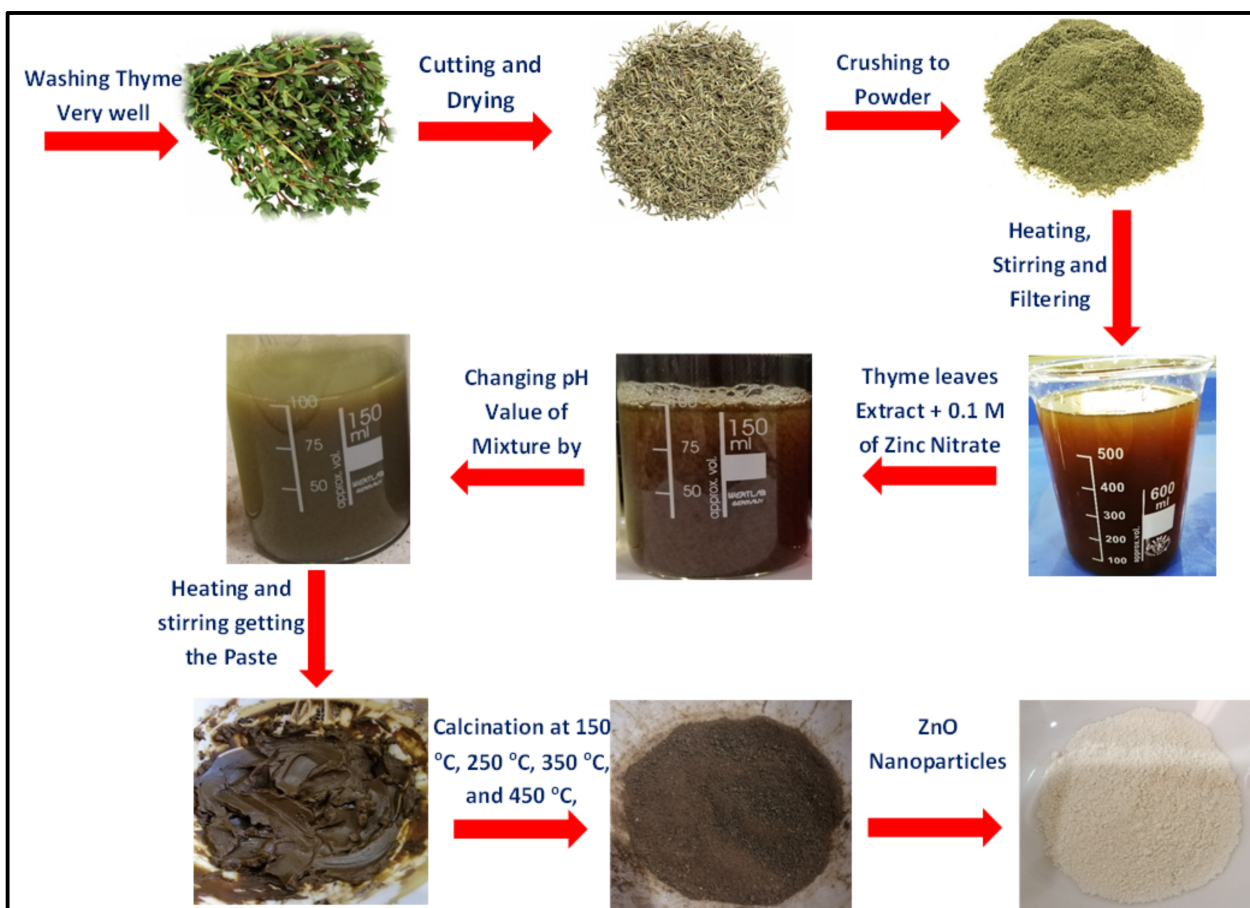
Figure 1. Schematic representation of green synthesis process of ZnO NPs by using the leaf extract of thyme plant and zinc nitrate hexahydrate.
