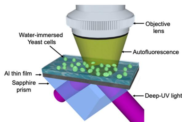
**Figure 1.** Schematic diagram of living yeast cell observation using deep-UV SPR.
