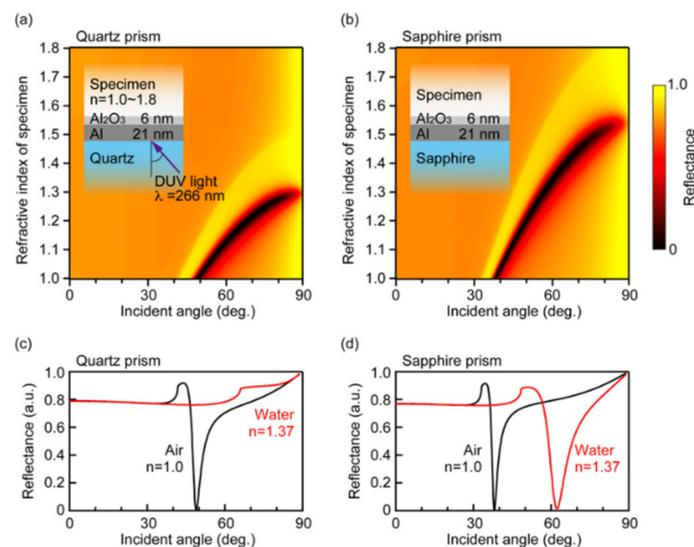
**Figure 2.** The theoretical reflectance dependence on the incident angle and the refractive index of specimen for aluminum thin film on (a) quartz and (b) sapphire prisms and the line profiles in refractive indices of air and water on (c) quartz and (d) sapphire prisms.
