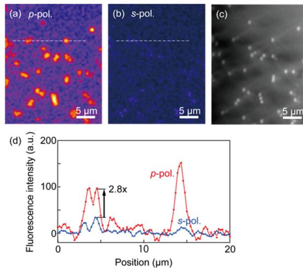
**Figure 4.** The fluorescence images of water-immersed polystyrene latexes excited with (a) *p*-polarization, (b) *s*-polarization, (c) conventional reflection image and (d) the fluorescence intensity line profiles between *p*-polarization and *s*-polarization fluorescence images.
