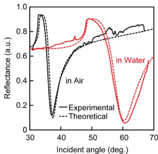
**Figure 3.** Experimental (solid) and theoretical (broken) reflectance dependences on the incident angle in air and in water.
