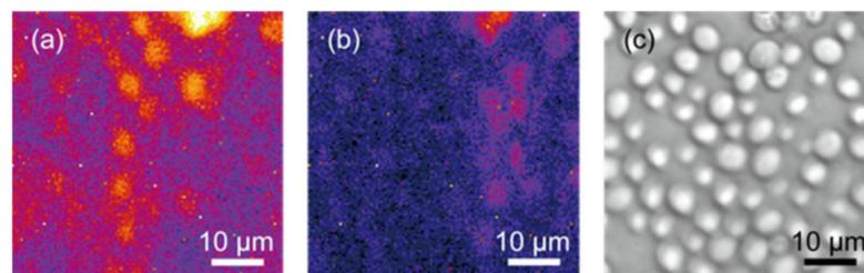
**Figure 5.** Water-immersed living yeast cells autofluorescence images on the aluminum thin film (a) with deep-UV SPR of *p*-polarization, (b) without deep-UV SPR of *s*-polarization and (c) conventional reflection image.
