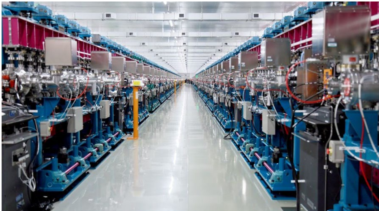
Figure 6. SACLA undulator hall: Two rows of ~100-m in-vacuum undulators producing XFEL. Left: BL3, right: BL2.
