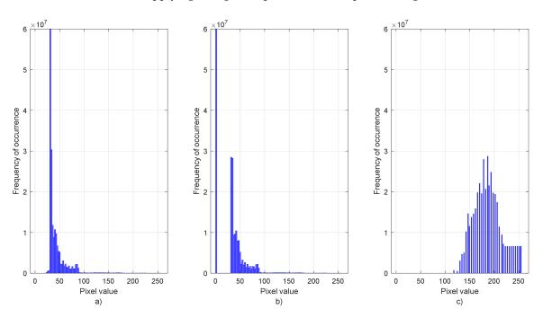
**Figure 4.** (a) Original histogram of grayscale image, (b) Histogram with background set to 0, and (c) Equalized histogram.
