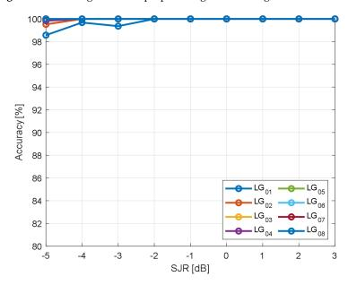
Figure 9. Accuracy of LG modes classification.
