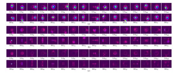
**Figure 2.** Measured beam profiles under jamming effect at SJRs of: (a) -5 dB, (b) 0 dB, and (c) 3 dB. Reprinted from ref. [14].
