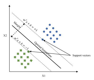
Figure 7. Illustration of binary SVM classifier.
