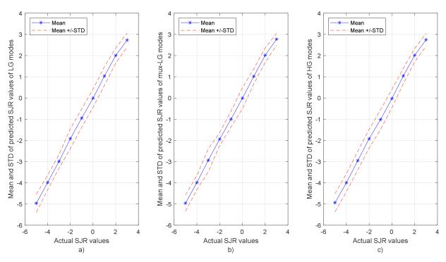
**Figure 17.** Mean  $\pm$  STD of estimated SJR values over fifty independent runs for: (a) LG, (b) Mux-LG, and (c) HG transmissions.
