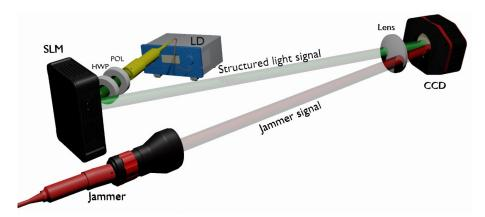
**Figure 3.** Conceptual block diagram of experimental setup. LD: laser diode, POL: polarizer, HWP: half-wave plate, CCD: charge-coupled device, and SLM: spatial light modulator.
