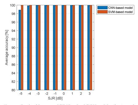
**Figure 12.** Results of the proposed SVM-Based and CNN-based classification methods when Mux-LG modes are considered.
