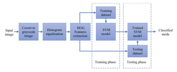
$\textbf{Figure 8.} \ \textbf{Block diagram of the proposed algorithm for light beam mode classification}.$
