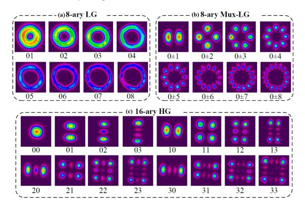
**Figure 1.** Experimentally generated beam profiles of: (a) LG, (b) Mux-LG, and (c) HG modes with no jamming interference. Reprinted from ref. [14].
