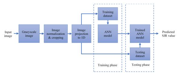
Figure 15. Block diagram of SJR estimation algorithm.
