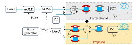
setup, the interrogator is divided into an in-house part and an on-site part, and the CIR is moved to the on-site part from the interrogator.
