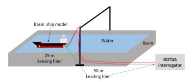
**Figure 1.** Schematic diagram of experimental setup for monitoring the dynamic strain of the basin ship model.
