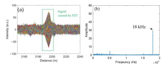
**Figure 4.** Experimental results of using the proposed  $\phi$ -OTDR setup. (a) Measured correct  $\phi$ -OTDR traces corresponding to the 2.19 km SF while filtering out the low-frequency components when the pulse repetition rate was 40 kHz, the location of PZT zone on the SF was the same as that in Figure 3a. (b) Frequency spectrum of the measured signal located at 2195 m (the same location as Figure 3b, 2195 m + LF = 12,445 m) within the PZT zone.
