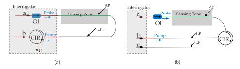
**Figure 7.** Comparison between the conventional and our proposed BOTDA systems when the interrogator is close to the sensing zone. Points "a", "b" and "c" represent the connection points. (a) Conventional BOTDA system, in which the OI and CIR are integrated into the interrogator. (b) By using our proposed approach, the OI and CIR are installed on-site. OI: optical isolator; CIR: circulator.
