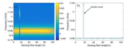
**Figure 6.** Experimental results of using the proposed BOTDA setup. (**a**) Measured BGS distribution along the sensing fiber. (**b**) Extracted strain distribution along the sensing fiber.
