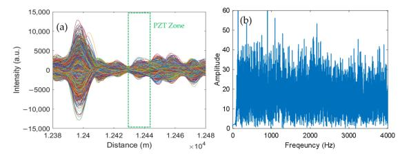
**Figure 3.** Experimental results of using conventional  $\phi$ -OTDR setup, the total length of the FUT was about 12.5 km. (a) Measured incorrect  $\phi$ -OTDR traces while filtering out the low-frequency components when the pulse repetition rate was 40 kHz. (b) Frequency spectrum of the measured incorrect signal located at 12,445 m, which was within the PZT zone.
