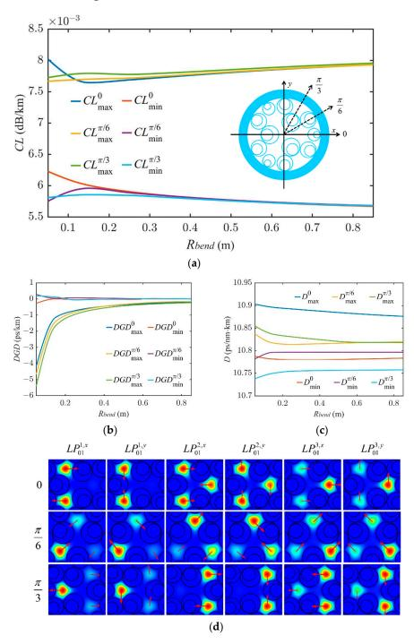
**Figure 11.** (a) Change in CL with the bending radius; (b) Change in DGD with the bending radius; (c) Change in D with the bending radius; (d) Electric field distribution of six fundamental supermodes when the bending radius is 0.05 m at three angle conditions (0,  $\pi/6$ , and  $\pi/3$ ), the direction of red arrows represents the direction of the electric field.
