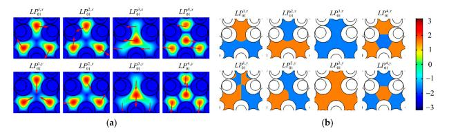
**Figure 2.** (a) Fundamental supermode electric field distribution of the four-core strongly coupled anti-resonant fiber, the direction of red arrows represents the direction of the electric field; (b) Fundamental supermode phase distribution of the four-core strongly coupled anti-resonant fiber and its color legend.
