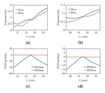
**Figure 8.** (a) Change in D with  $r_1$ ; (b) Change in D with  $r_2$ ; (c) Change in DGD with  $r_1$ ; (d) Change in DGD with  $r_2$ .
