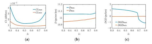
**Figure 16.** (a) Change in CL in the new structure with  $k_1$ ; (b) Change in D in the new structure with  $k_1$ ; (c) Change in DGD in the new structure with  $k_1$ .
