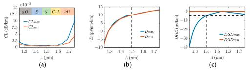
**Figure 13.** (a) CL of the change in TCS-ARF with  $\lambda$ . (b) D of the change in TCS-ARF with  $\lambda$ . (c) DGD of the change in TCS-ARF with  $\lambda$ .
