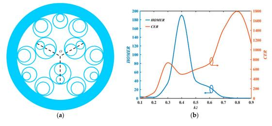
**Figure 15.** (a) The previous structure with the addition of a tube; (b) the change in HOMER and CER with  $k_2$ .
