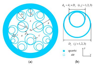
**Figure 1.** (a) Schematic diagram of the NMH-ARF structure; (b) Schematic diagram of the nested capillary structure.
