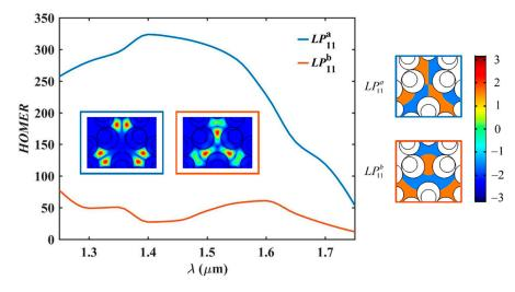
**Figure 14.** The change in HOMER with  $\lambda$ . The two most representative electric field distributions of the high-order supermodes  $LP_{11}^a$  and  $LP_{11}^b$  are on the left, and their corresponding phase distributions are on the right. The color legend is for the phase distributions.
