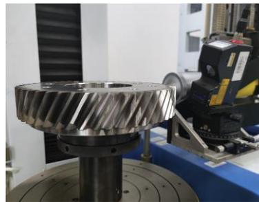
**Figure 6.** Gear measurement process.
