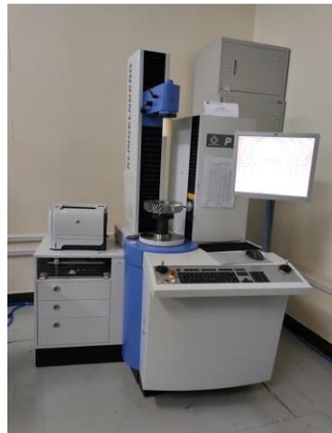
Figure 11. Gear measurement center (P26, Klingelberg, Ettlingen, Germany).
