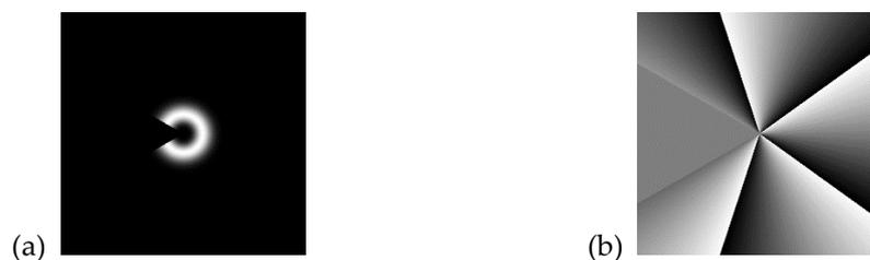
**Figure 3.** An amplitude (a) and phase (b) of the incident field at  $\alpha = 150^\circ$ ,  $20 \times 20$   $\mu\text{m}$ , TC  $m = 5$ .
