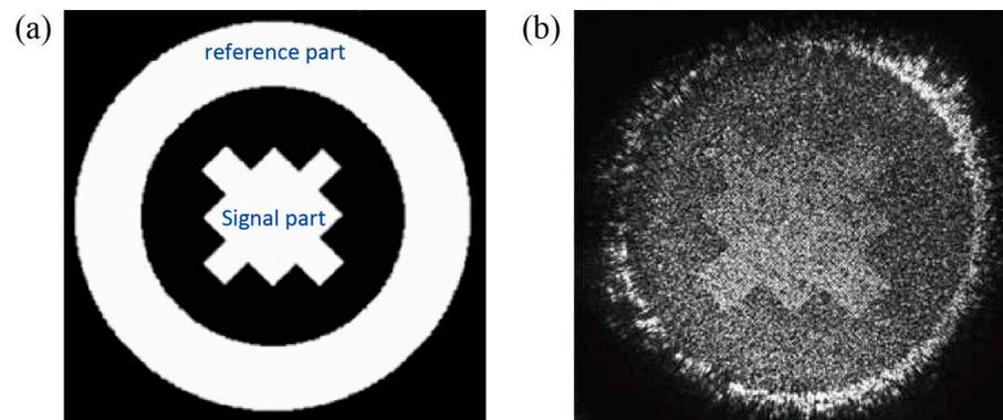
**Figure 4.** The signal image of magnetic hologram. (a) Recording pattern of the collinear hologram and (b) reconstruction of the signal image [24].
