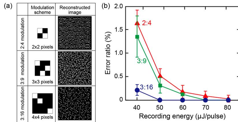
**Figure 5.** (a) Modulation schemes and example of reconstructed images recorded at 80 μJ encoded with 2:4, 3:9, and 3:16 modulation schemes. Each reconstructed signal pattern consists of 64 × 64 pixels. (b) The error ratio in reconstructed images for the three modulation schemes [30].
