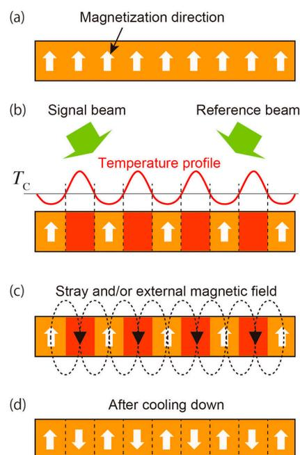
**Figure 2.** Schematics of recording process of magnetic hologram. (a) Perpendicularly magnetized recording medium. (b) As the result of interference, the medium is locally heated up higher than Curie temperature,  $T_C$ , by the absorption of light. (c) The magnetization of the heated region is reversed by stray and/or external magnetic fields during cooling. (d) The interference pattern of light can be recorded as the difference in the direction of magnetization.
