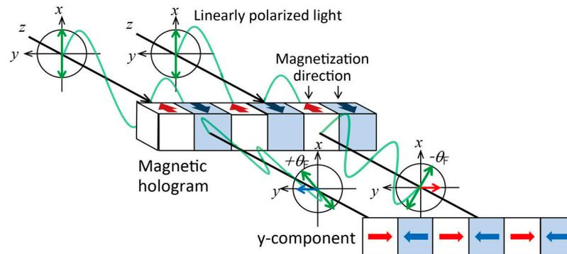
Figure 3. Principle of the reconstruction of magnetic hologram.
