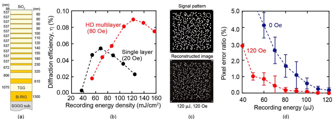
**Figure 10.** (a) Designed structure of HD multilayer medium; (b) diffraction efficiency of HD multilayer and single layer media; (c) original signal pattern and reconstructed image from HD multilayer medium. The signal pattern consists of  $64 \times 64$  pixels; (d) pixel error ratio of the reconstructed signal with and without the assisted magnetic field [33].
