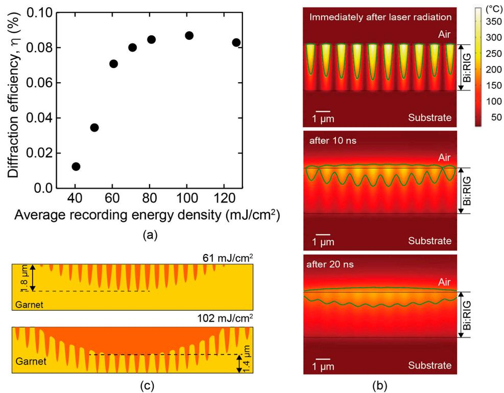
**Figure 7.** (a) Calculated diffraction efficiency at 1500 line-pairs/mm. (b) Calculated variation in temperature distribution around the garnet layer after laser irradiation with 81 mJ/cm<sup>2</sup>. The shape of the regions with a temperature higher than the Curie temperature (150 °C) is surrounded by green line. (c) Calculated shapes of obtained magnetic fringes in garnet recorded at 61 mJ/cm<sup>2</sup>, and 102 mJ/cm<sup>2</sup> [33].
