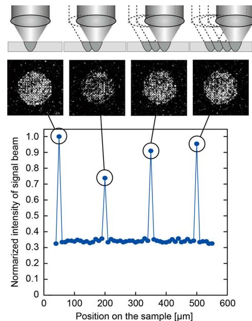
**Figure 6.** Results of shift multiplex recording of a magnetic collinear hologram showing schematic recording positions of the shift multiplex recording, and the intensity of the signal light and the corresponding reconstructed image plotted against the position on the sample [24].
