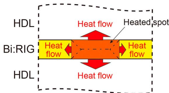
**Figure 8.** Concept of heat dissipation layer. Most of excess heat in Bi:RIG magnetic layer is diffused into HDLs to reduce heat diffusion in Bi:RIG.
