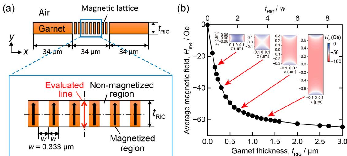
**Figure 9.** Calculated stray magnetic field in the magnetic fringe: (a) Calculation model and (b) the calculated average stray magnetic field along the center of a non-magnetized region and the stray magnetic field distributions in a non-magnetized region at several aspect ratios (inset). Negative values of magnetic field mean that the direction of the magnetic field is opposite to the initial direction [32].
