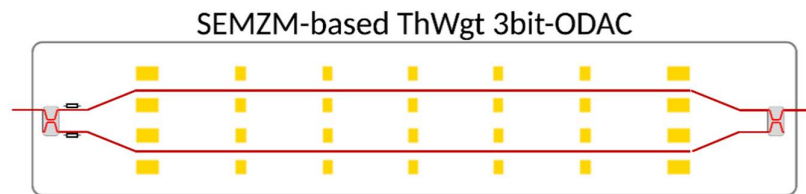
Figure 1. Segmented MZM (SEMZM) 7 segments oDAC architecture-optimized Thermometer-Weighted (ThWgt) DAC structure for generation of PAM8. The S = 7 electrode segment lengths are shown to scale for ThWgt operation (generation of an equi-spaced C = 8 -levels constellation). The guard spaces between segments not shown to scale.
