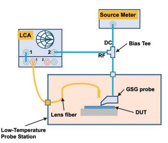
**Figure 6.** Bandwidth characterization of high-speed photodetector with Lightwave Component Analyzer (LCA).
