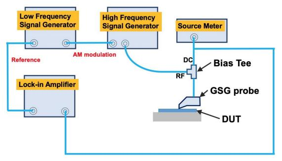
Figure 8. The schematics of the microwave rectification setup.
