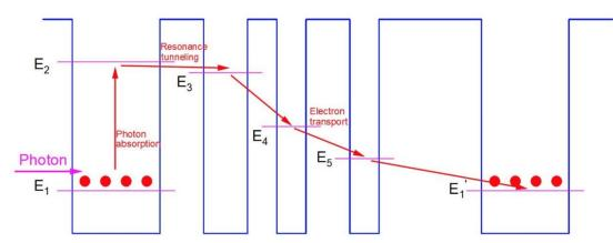
**Figure 3.** Conduction band of quantum cascade photodetectors. Reproduced from Ref. [32], with permission of AIP Publishing.
