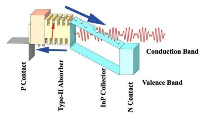
Figure 5. The schematics of the band diagram of the 2  $\mu$ m UTC photodiodes with type-II MQW as the absorber.
