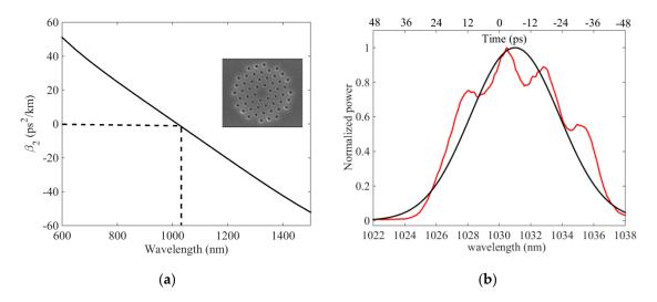
**Figure 1.** (a) Second order dispersion term as a function of the wavelength. Inset. Input facet of the PCF measured with a scanning electron microscope. (b) Normalized pump spectrum of a chirped pulse with a Gaussian shape (black line) or with the experimental profile (red line).
