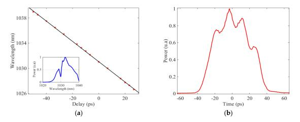
**Figure 5.** (a) Measurement of the chirp rate by spectral interferometry and its linear fit leading to  $\alpha = 6.2 \text{ ps/nm}$ . The inset is an example of the interference pattern. (b) Temporal shape of the pump pulse.
