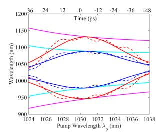
**Figure 2.** Phase matching as a function of the pump wavelength for a chirped pulse with a Gaussian spectrum (solid red and blue lines) or with the experimental profile (dashed red and blue lines). The maximum power was 600 W (red lines) or 200 W (blue lines). The magenta and cyan lines correspond to the phase matching for a constant peak power of 600 W or 200 W, respectively.
