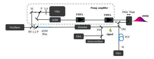
**Figure 3.** Experimental set-up. VBG, volume Bragg grating; AOM, acoustooptic modulator; YDFA, ytterbium doped fiber amplifier; OSA, optical spectrum analyzer; PCF, photonic crystal fiber; ANDI, all normal dispersion fiber; BS, beam splitter; M, mirror; P, polarizer; DM, dichroic mirror; FM, flipped mirror.
