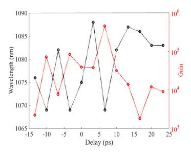
**Figure 7.** Maximum gain value (red circles) and its corresponding signal wavelength (black circles) as a function of the delay.
