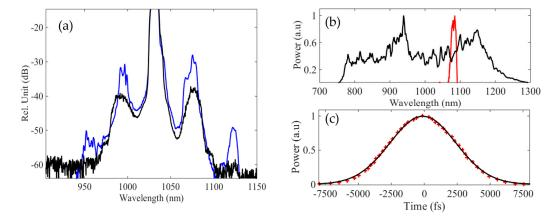
**Figure 4.** (a) Fluorescence spectrum when the PCF is pumped by 31 mW (black line). Output spectrum when the signal is injected at null delay (blue line). (b) Spectrum of the continuum generated in the ANDI fiber (black line) and spectrum of the signal (red line). (c) Autocorrelation trace (red stars) and the Gaussian fit (solid black line) of the signal.
