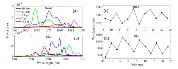
**Figure 6.** (**a**,**b**) Selection of amplified and idler spectra when the delay is tuned from -6.6 ps to +19.8 ps. (**c**,**d**) Variation of the signal and idler wavelengths at the maximum amplification as a function of the delay.
