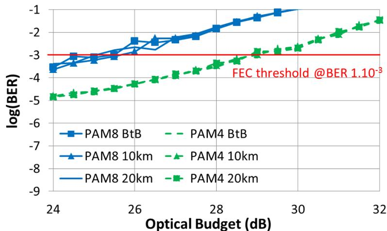
**Figure 7.** BER of 37.5 Gbit/s PAM8 and 50 Gbit/s PAM4 versus Optical Budgets for 0, 10, and 20 km.
