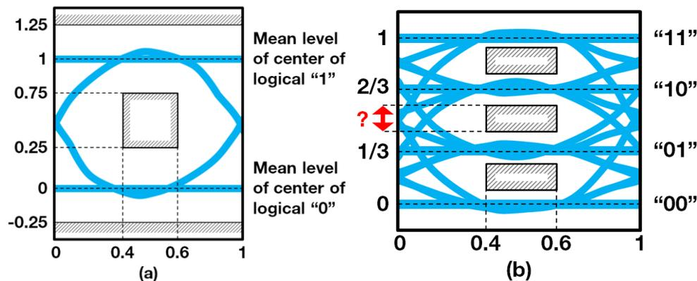
**Figure 3.** Mask of the eye diagram for OLT transmitter (a) and proposition for PAM (b).
