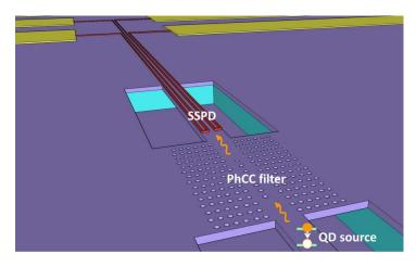
**Figure 1.** Sketch of the proposed approach for the quantum photonic integrated circuits (QPIC). Single photons are produced via spontaneous emission of excitons in quantum dots (QDs), efficiently funneled in waveguides, filtered by a photonic crystal cavity (PhCC) and detected by waveguide superconducting single photon detectors (SSPDs).
