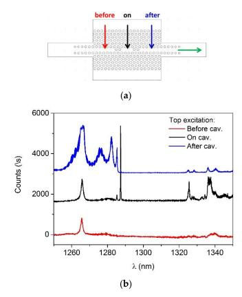
**Figure 8.** (a) Sketch of the design B filter: the red (before cavity), black (on cavity), and blue (after cavity) arrows indicate the different position of the top excitation, while the green the direction of the side collection. (b) PL spectra for the three different excitation positions with color coding corresponding to (a). The blue spectra has been reduced by a factor of 5 for greater clarity.
