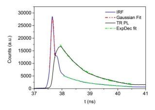
**Figure 6.** Instrument response function (IRF) of the SSPD (blue) and on-chip time resolve QD photoluminescence measurement (black). The red line represents the Gaussian fit of the IRF and the green lines the exponential fit of the decay time of the QD emission.
