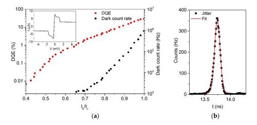
**Figure 4.** (a) Device quantum efficiency (DQE) (red) of a 20  $\mu$ m-long SSPD on top of SNB under illumination at 1300 nm, and dark count rate (black) as a function of the normalized bias current. Inset: current-voltage characteristic. (b) Histogram of the jitter time of the detector biased 94% *I*<sub>c</sub>.
