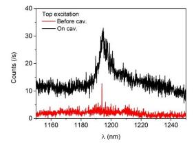
**Figure 10.** PL spectra on two different excitation position following the previous color coding. A single QD excitonic line is clearly visible on the red curve.
