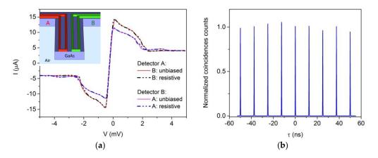
**Figure 5.** (a) I-V curve of Detector A while Detector B is unbiased or in resistive state; I-V curve of Detector B while Detector A is unbiased or in resistive state. Inset: sketch of the two independent SSPDs on top of SNB. (b) Coincidence rate under illumination with a 80 MHz pulsed laser at 965 nm and detectors biased at 97%  $I_c$ .
