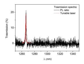
**Figure 9.** Experimental transmission spectra: black curve indirectly calculated from the ratio between the photoluminescence (PL) spectra before and after filtering, red curve from direct fiber-in:fiber-out measurement.
