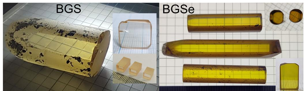
**Figure 1.** Images of boules, elements, and plates of BGS and BGSe crystals grown by the Bridgman–Stockbarger technique.
