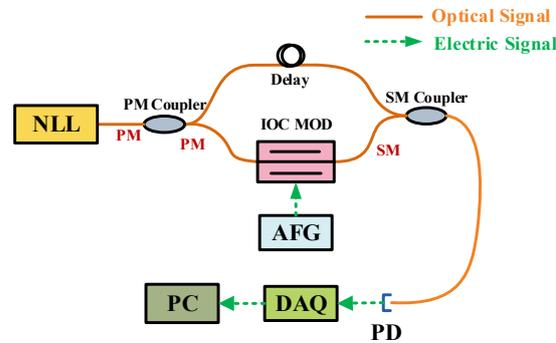
Figure 6. Schematic of experiment setup for phase-generated carrier signal measurement.
