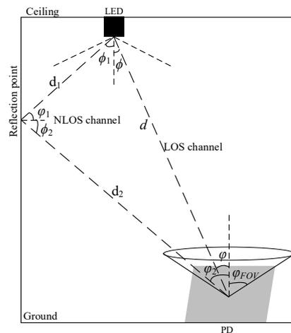
Figure 2. Indoor visible light channel.
