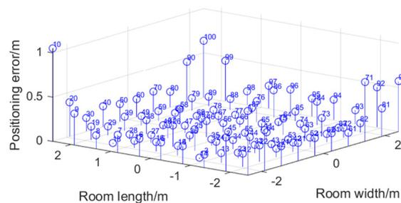
**Figure 8.** Location error using the fingerprint method.
