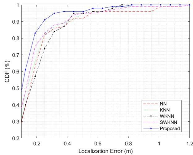
Figure 12. Cumulative probability of errors in different algorithms.
