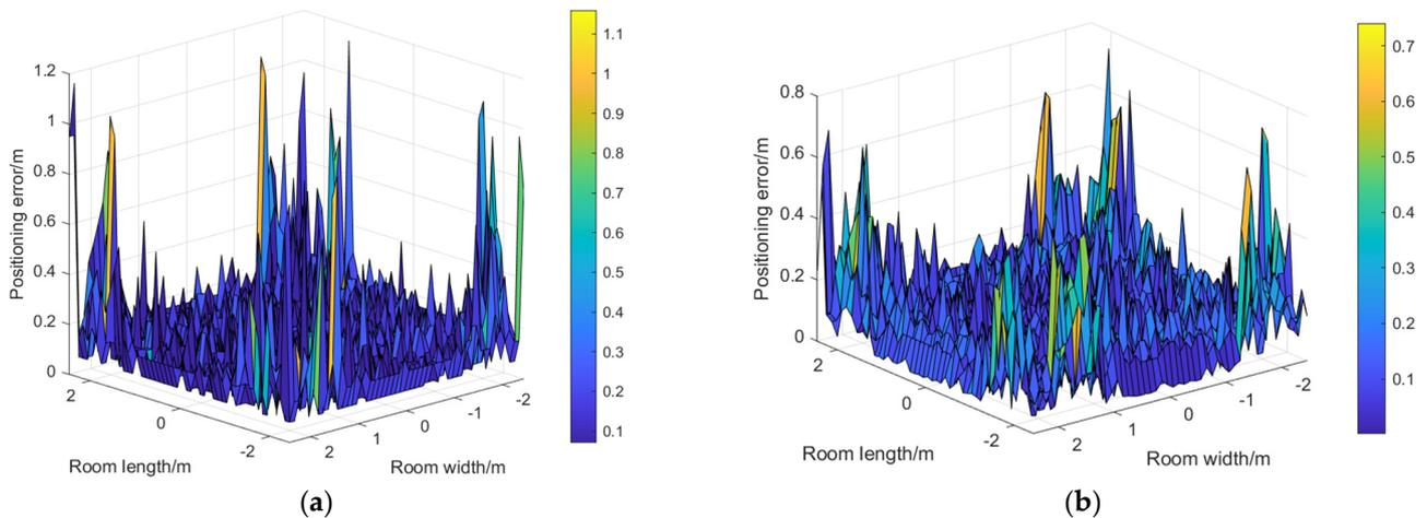
**Figure 11.** Location error distribution diagram. (a) Traditional fingerprint method; (b) proposed algorithm.
