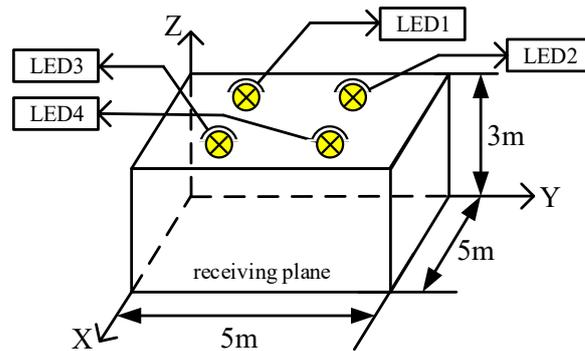
Figure 1. Indoor VLC system model.
