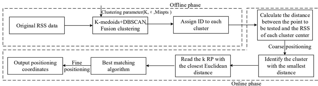
Figure 4. Indoor positioning system based on fingerprint.
