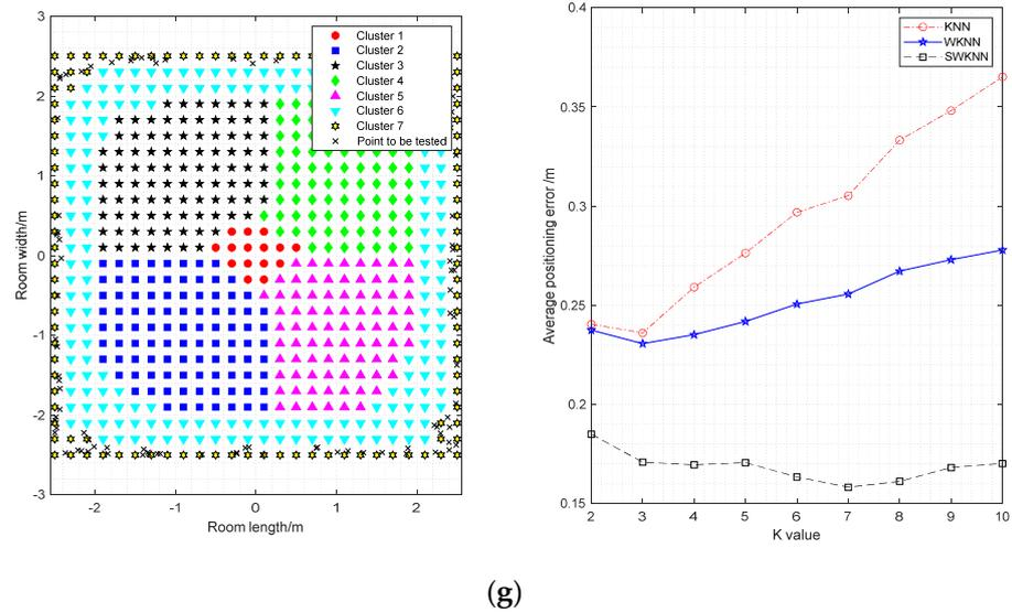
**Figure 10.** Clustering effect diagram and positioning error of each region: (a) Cluster 1; (b) cluster 2; (c) cluster 3; (d) cluster 4; (e) cluster 5; (f) cluster 6; (g) cluster 7.
