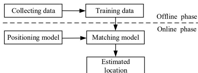
Figure 3. Indoor positioning system based on fingerprint.
