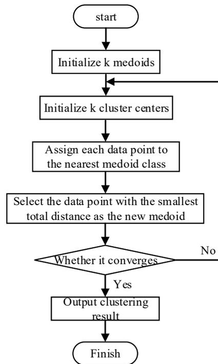
Figure 5. K-medoids clustering algorithm flow chart.
