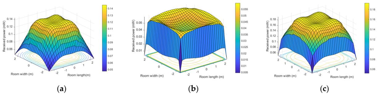
**Figure 7.** Distribution of received optical power: (a) LOS channel; (b) channel with only one reflection; (c) total channel.
