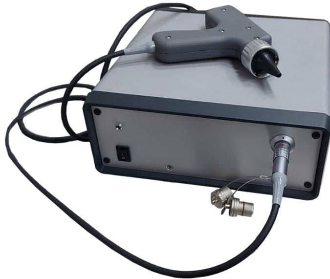
**Figure 1.** The base block and the handheld probe of the SDOCT otoscopic system.
