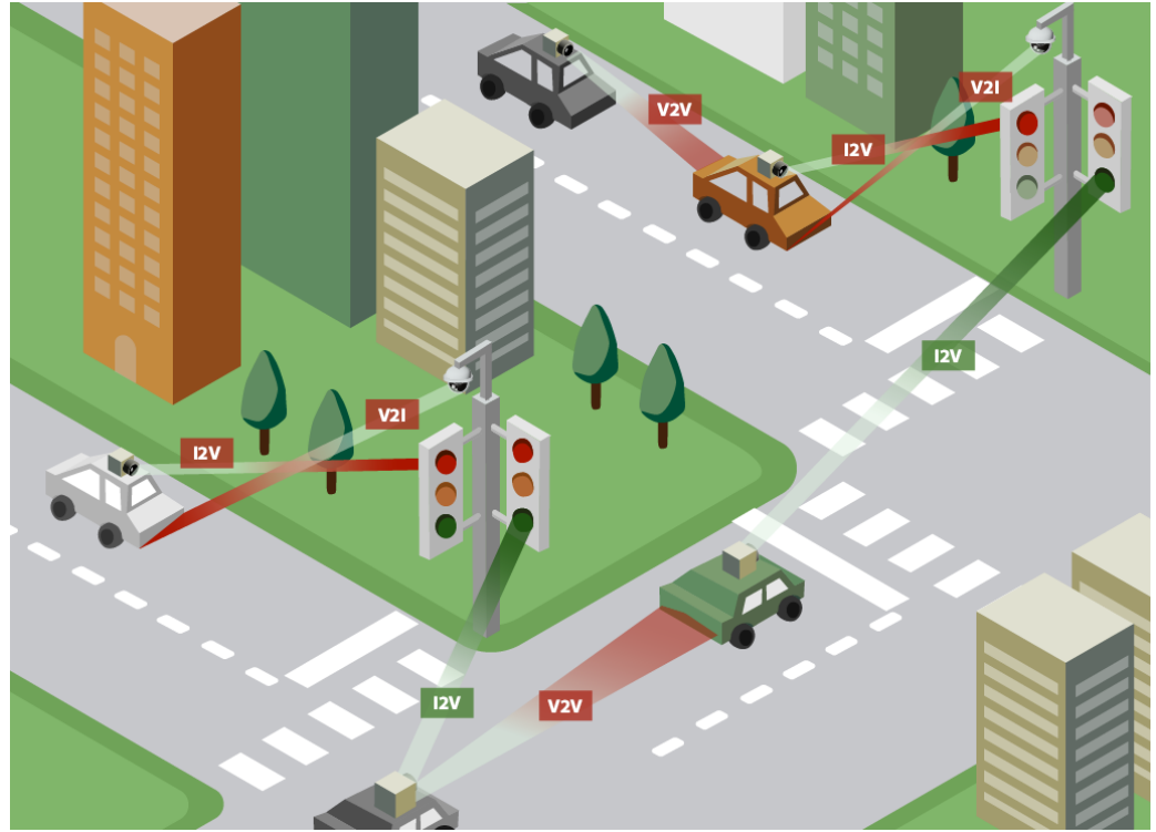
Figure 6. The basic idea of image sensor communication for vehicular applications including vehicle-to-vehicle (V2V), vehicle-to-infrastructure (V2I), and infrastructure-to-vehicle (I2V) communications. Data signals are emitted from traffic lights and vehicle headlights and taillights. Image sensors are mounted on the vehicle to receive visible light signals. The image sensor converts the received visible light signal into an electrical signal and decodes the signal using image processing technology.
